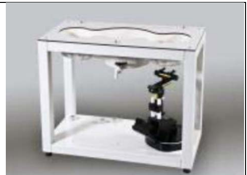
Fig. 6.8 Photo of SAM Phantom
