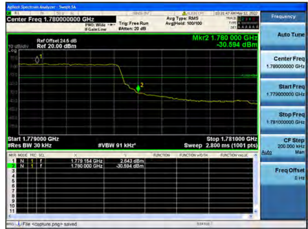
Band66 / 1.4MHz / High CH / QPSK / FULL RB
