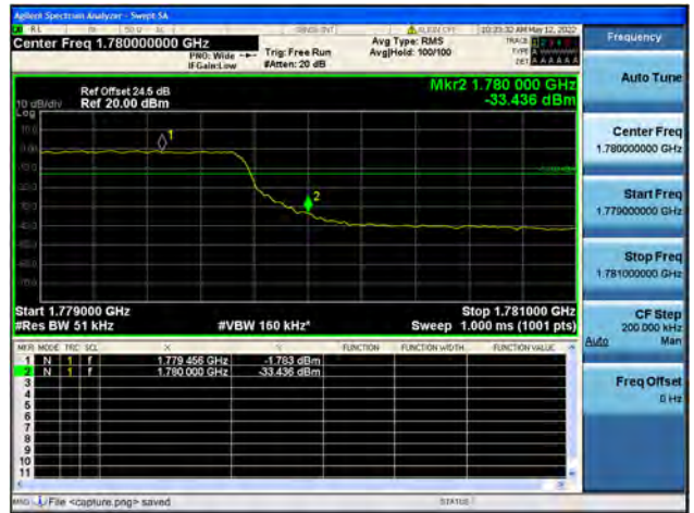
Band66 / 5MHz / High CH / QPSK / FULL RB
