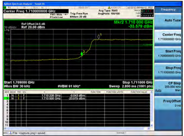
Band66 / 3MHz / High CH / QPSK / FULL RB
