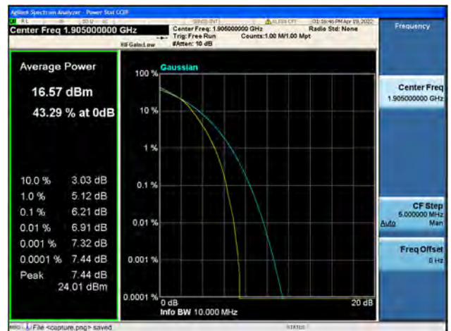
Band2 / 10MHz / High CH / 64QAM
