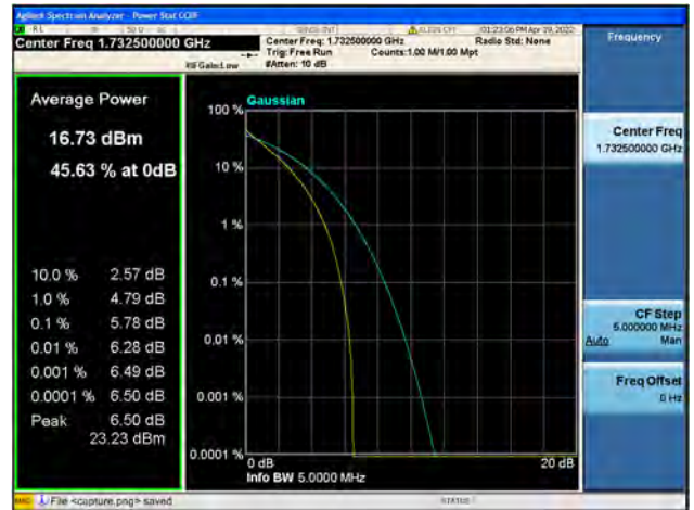
Band4 / 1.4MHz / Mid CH / 64QAM
