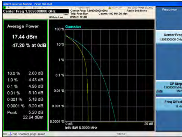
Band2 / 1.4MHz / High CH / 64QAM
