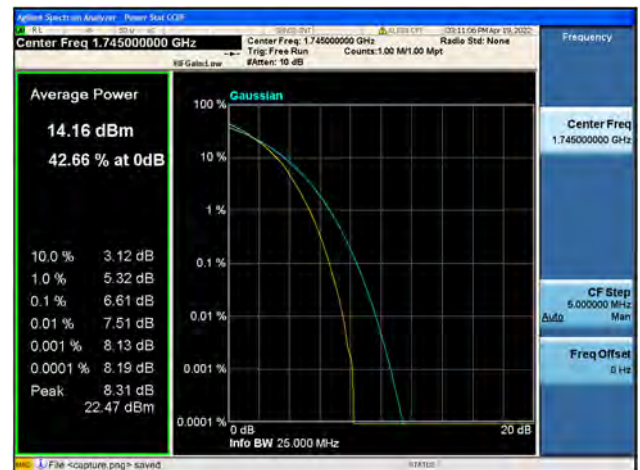
Band66 / 15MHz / Mid CH / 64QAM
