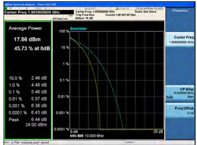
Band2 / 10MHz / High CH / 64QAM
