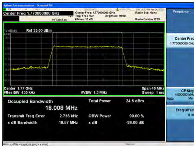
Band66 / 20MHz / High CH / 16QAM
