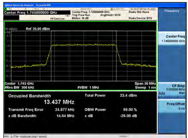
Band66 / 15MHz / Mid CH / 64QAM
