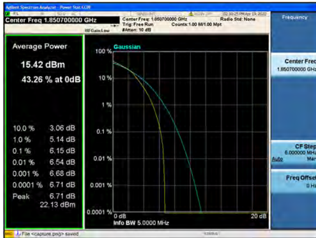
Band25 / 1.4MHz / Mid CH / 16QAM
