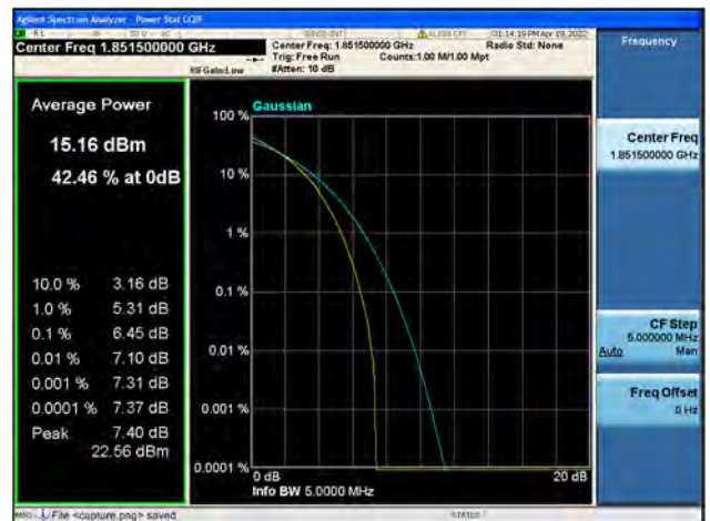
Band2 / 3MHz / Low CH / 64QAM
