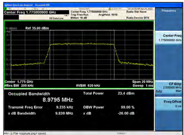
Band66 / 10MHz / High CH / 64QAM
