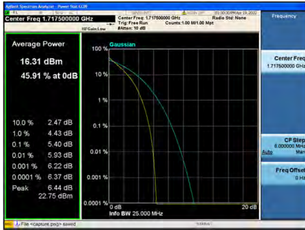
Band4 / 15MHz / Low CH / 64QAM
