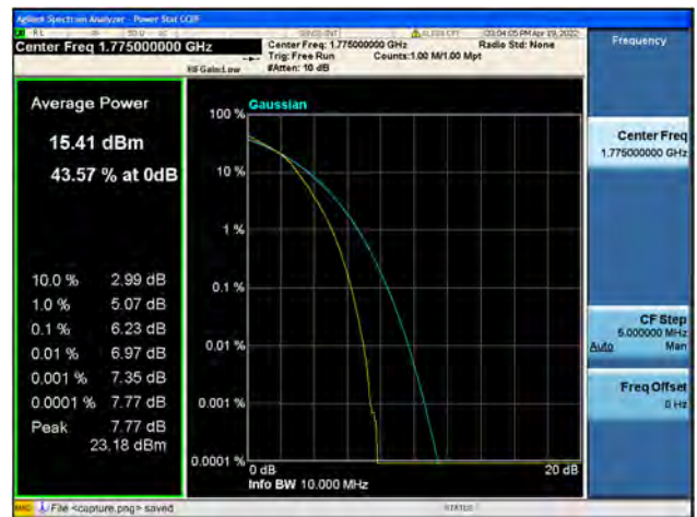
Band66 / 10MHz / High CH / 64QAM
