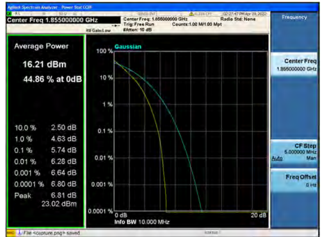
Band25 / 10MHz / Low CH / 64QAM
