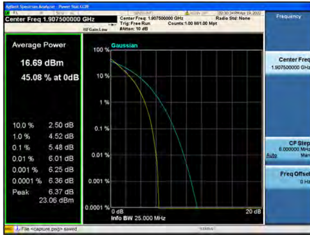
Band25 / 15MHz / High CH / 64QAM
