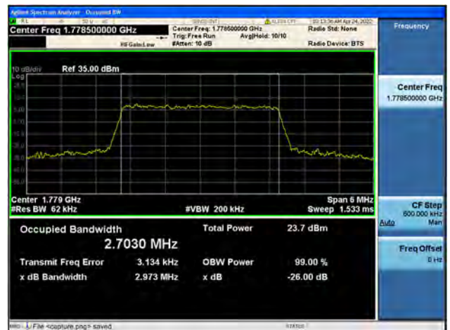
Band66 / 3MHz / High CH / 64QAM
