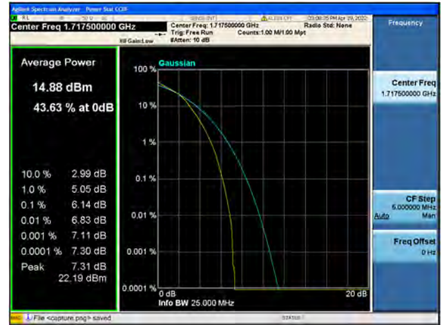
Band66 / 15MHz / Mid CH / QPSK
