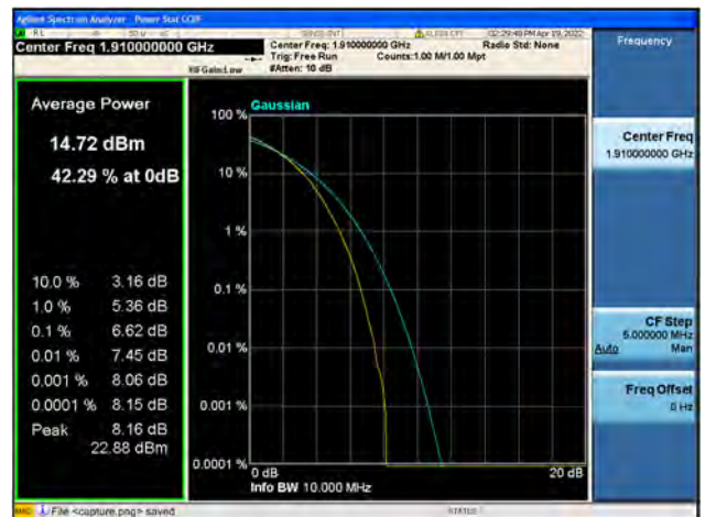
Band25 / 10MHz / High CH / 64QAM
