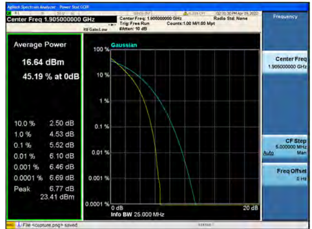
Band25 / 20MHz / High CH / 64QAM
