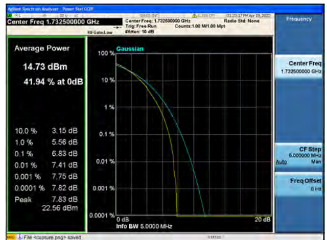
Band4 / 1.4MHz / Mid CH / 64QAM
