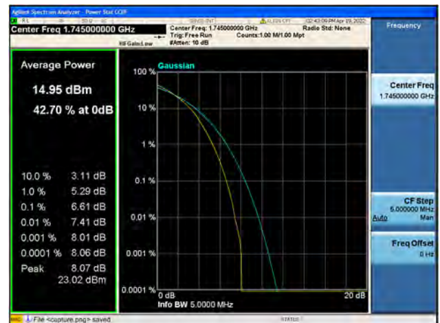
Band66 / 5MHz / Mid CH / 64QAM
