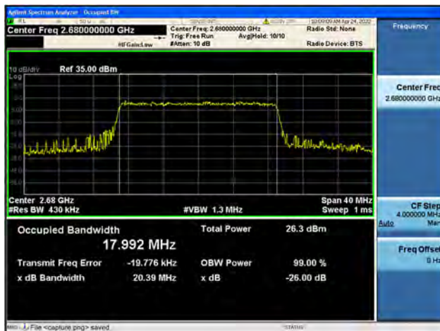
Band41 / 20MHz / High CH / 16QAM
