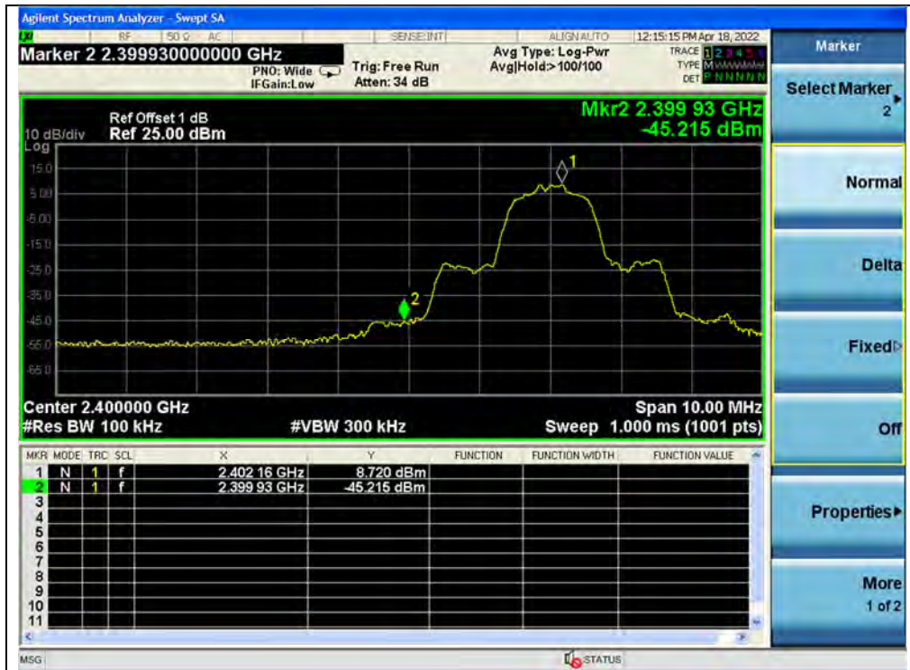
(Band edge, Channel 0, \pi/4 -DQPSK)
