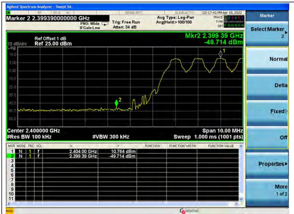
(Band edge with hopping on, Channel 0, GFSK)
