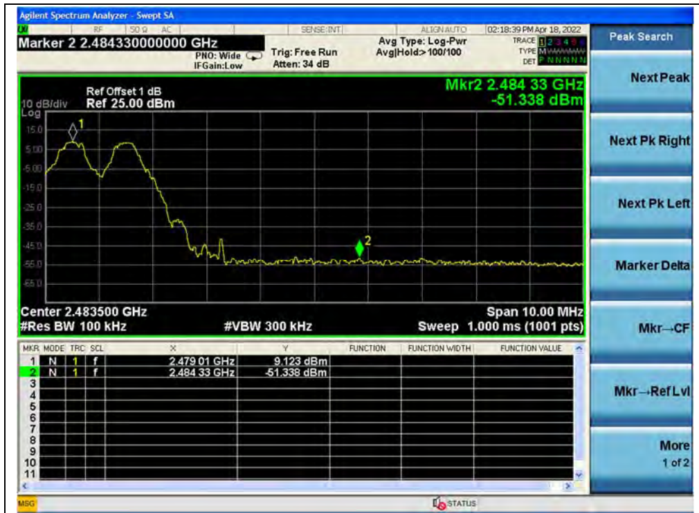
(Band edge with hopping on, Channel 78, GFSK)
