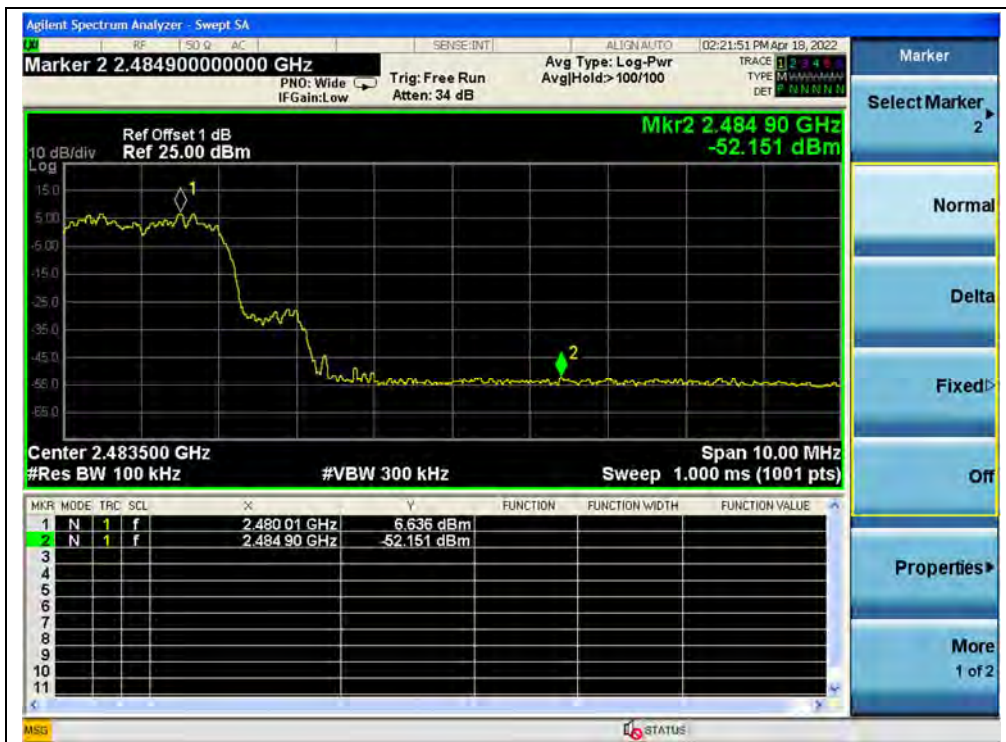
(Band edge with hopping on, Channel 78, 8-DPSK)
