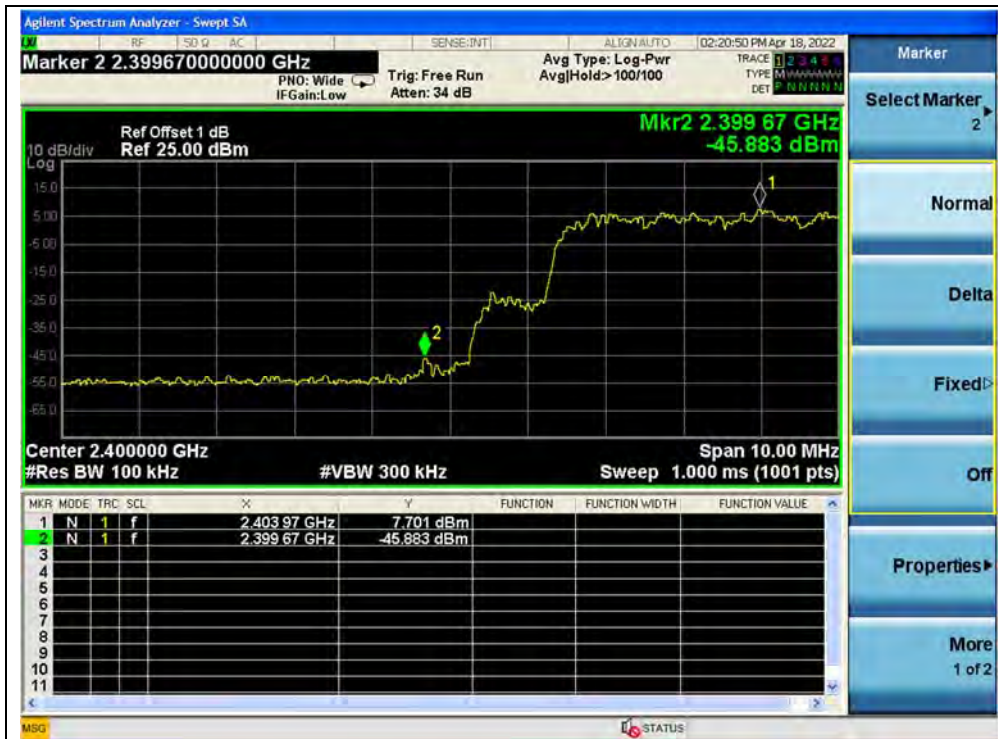
(Band edge with hopping on, Channel 0, 8-DPSK)
