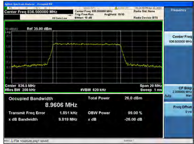
Band5 / 10MHz / High CH / QPSK
