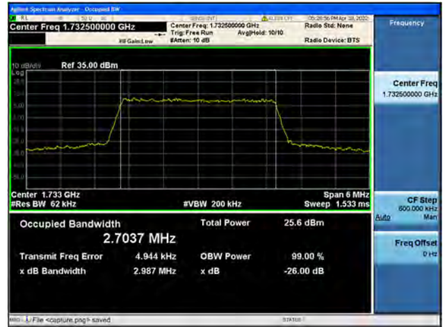
Band4 / 3MHz / High CH / QPSK
