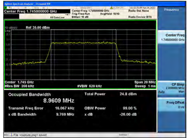
Band66 / 10MHz / High CH / QPSK
