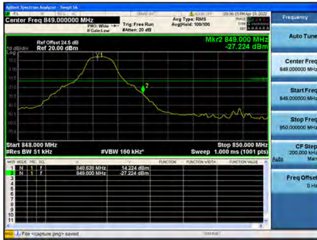
Band5 / 5MHz / High CH / QPSK / 1 RB
