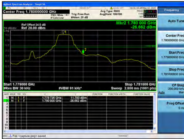
Band66 / 1.4MHz / High CH / QPSK / 1 RB
