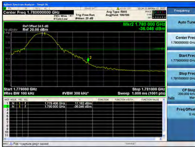
Band66 / 10MHz / High CH / QPSK / 1 RB
