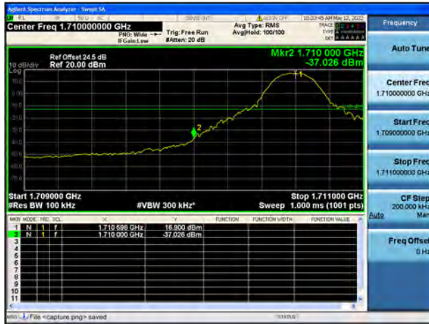
Band66 / 10MHz / High CH / QPSK / 1 RB
