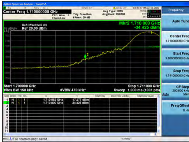
Band4 / 15MHz / High CH / QPSK / 1 RB
