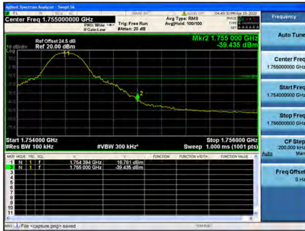
Band4 / 10MHz / High CH / QPSK / 1 RB
