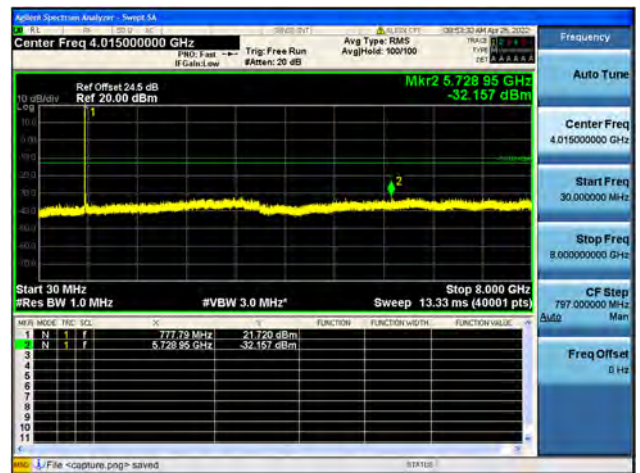
Band13 / 10MHz / High CH / 64QAM
