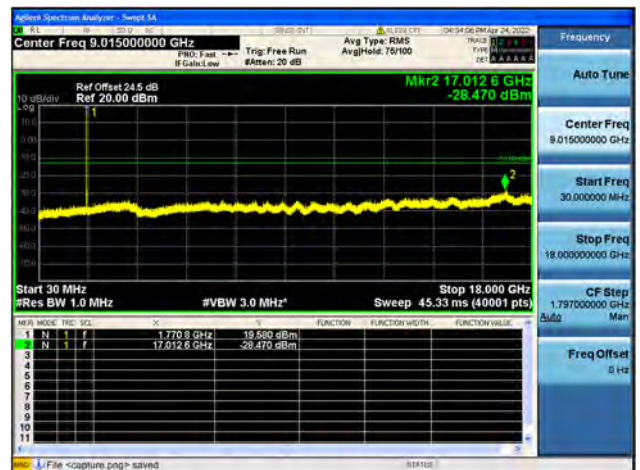
Band66 / 10MHz / High CH / 64QAM
