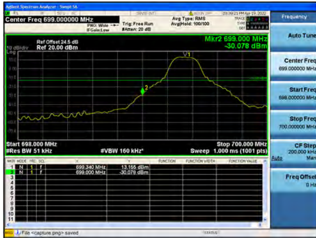
Band12 / 5MHz / High CH / QPSK / 1 RB
