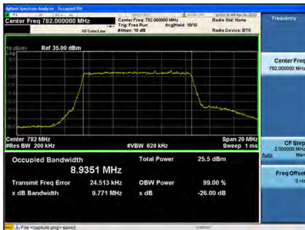
Band13 / 10MHz / High CH / 16QAM
