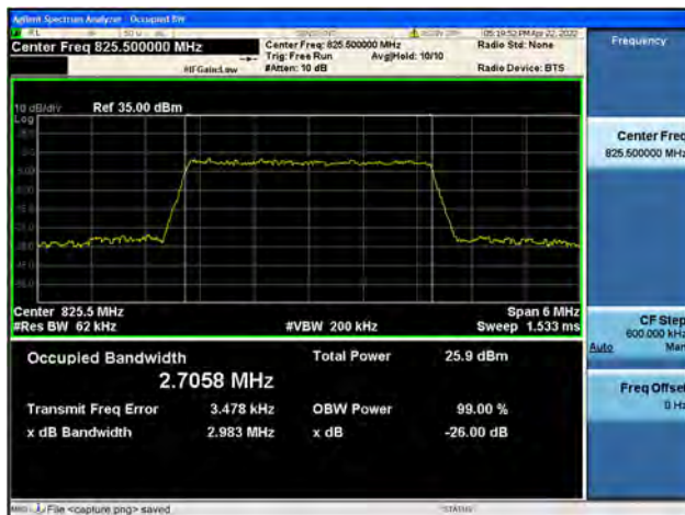
Band5 / 3MHz / Low CH / 16QAM
