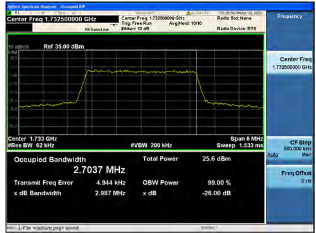
Band4 / 3MHz / High CH / QPSK
