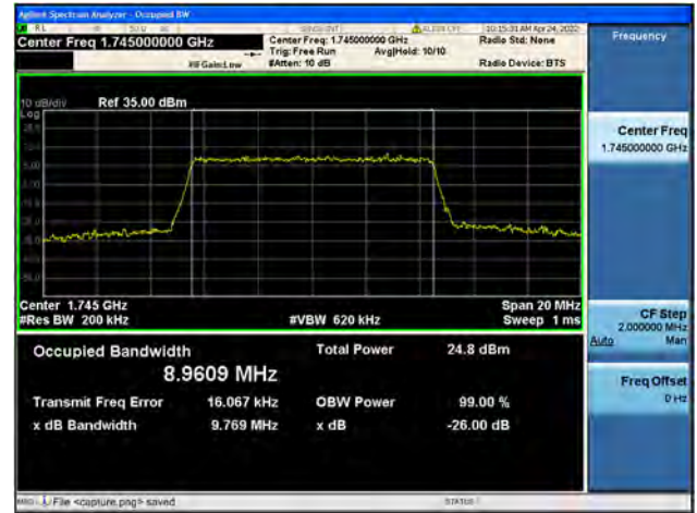
Band66 / 10MHz / High CH / QPSK
