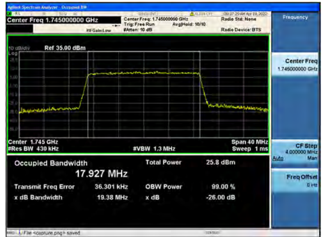
Band4 / 20MHz / High CH / 64QAM
