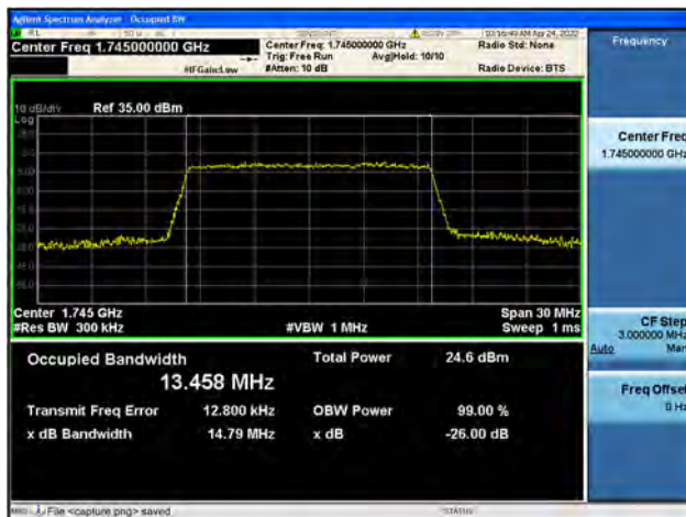
Band66 / 15MHz / Mid CH / 16QAM
