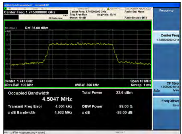
Band66 / 5MHz / Mid CH / 64QAM
