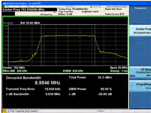
Band13 / 10MHz / High CH / 16QAM
