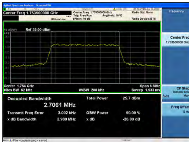
Band4 / 3MHz / High CH / 16QAM
