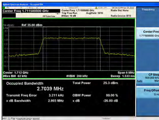
Band4 / 3MHz / Low CH / 16QAM
