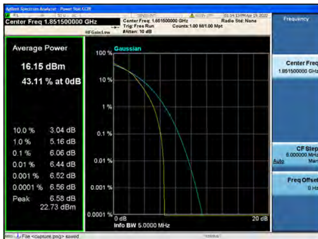
Band2 / 3MHz / Low CH / 16QAM
