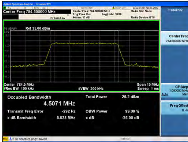
Band13 / 5MHz / High CH / 64QAM
