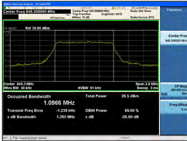
Band5 / 1.4MHz / High CH / 64QAM
