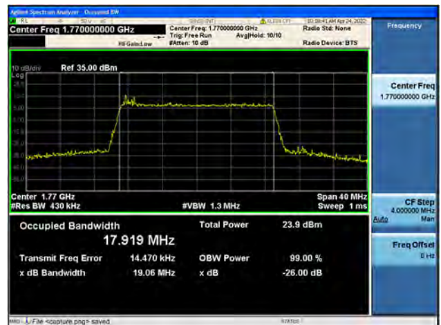
Band66 / 20MHz / High CH / 64QAM
