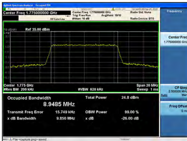
Band66 / 10MHz / High CH / 16QAM
