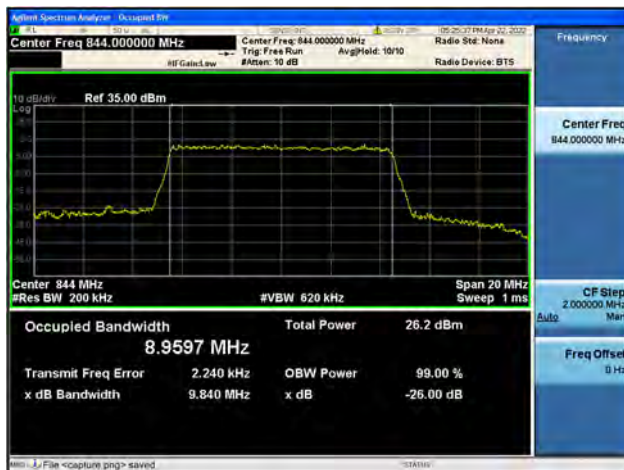
Band5 / 10MHz / High CH / 16QAM
