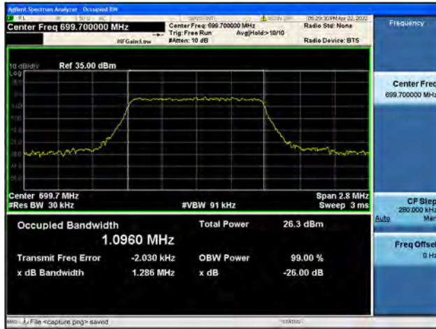
Band12 / 1.4MHz / Low CH / 64QAM
