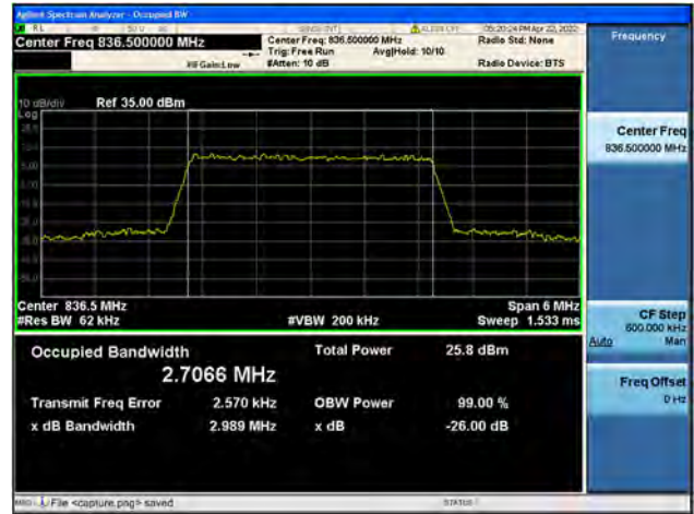
Band5 / 3MHz / High CH / QPSK
