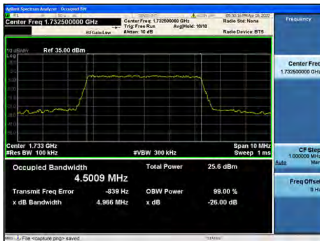
Band4 / 5MHz / Mid CH / 16QAM
