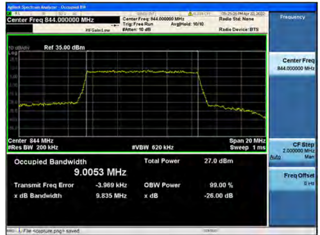
Band5 / 10MHz / High CH / 64QAM
