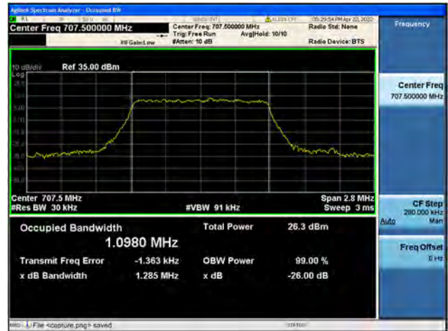
Band12 / 1.4MHz / Mid CH / 64QAM
