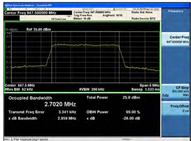
Band5 / 3MHz / High CH / 64QAM
