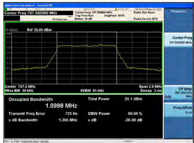
Band12 / 1.4MHz / Mid CH / 64QAM
