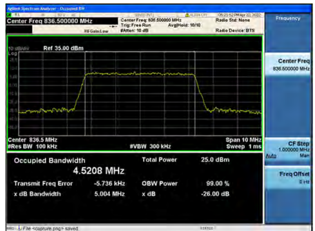
Band5 / 5MHz / Mid CH / 64QAM
