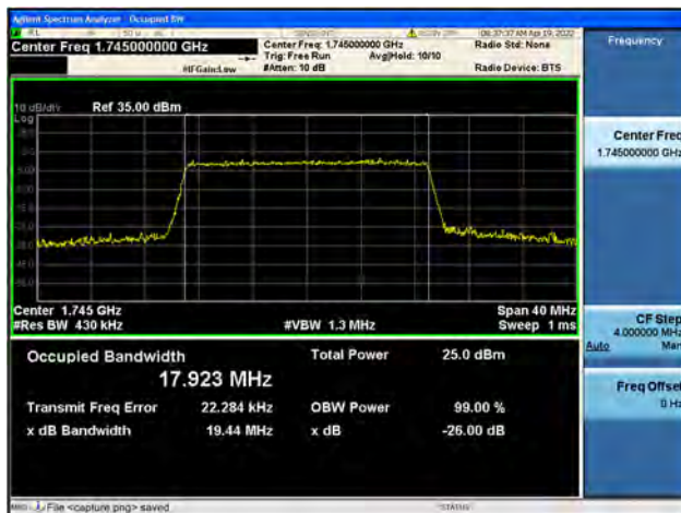
Band4 / 20MHz / High CH / 16QAM
