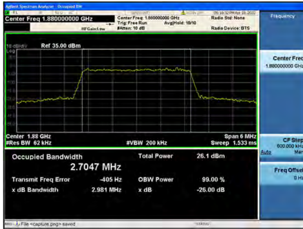
Band2 / 3MHz / Mid CH / 64QAM
