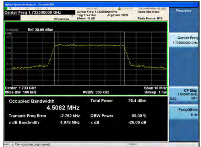
Band4 / 5MHz / Mid CH / 64QAM
