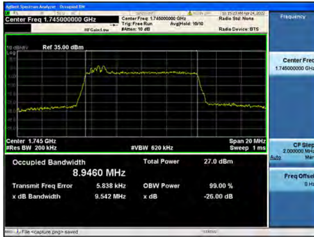
Band66 / 10MHz / Mid CH / 64QAM
