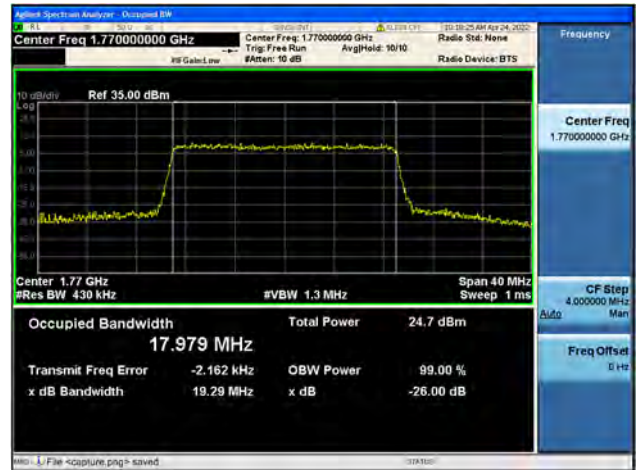
Band66 / 20MHz / High CH / 64QAM
