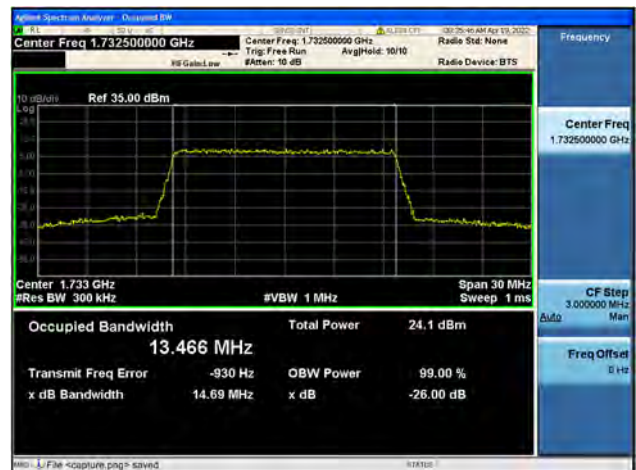
Band4 / 15MHz / Mid CH / 64QAM
