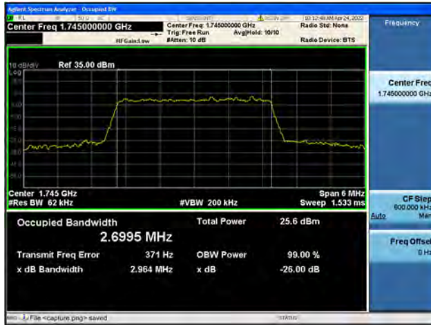
Band66 / 3MHz / Mid CH / 64QAM
