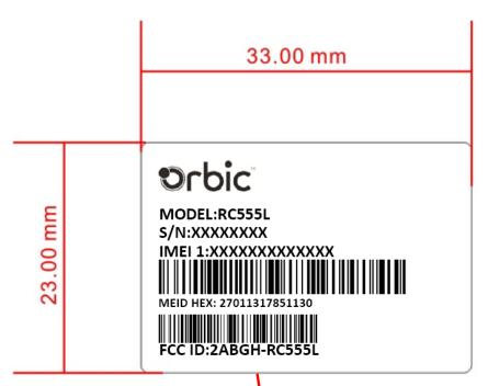
The label is inside the back cover, and the cover can be easily opened.
