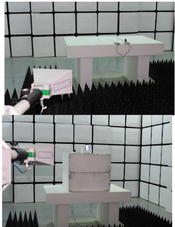
**1.3** Setup for Unwanted Emissions that fall Outside of the Restricted Bands(Radiated) and Unwanted Emissions in the Restricted Bands (Radiated) above 1GHz
