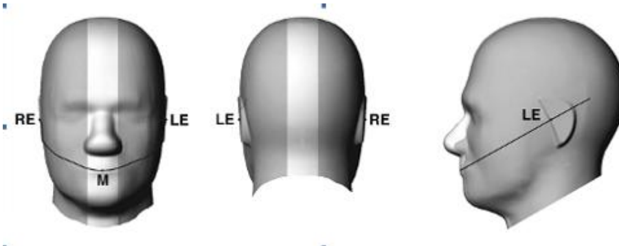
F-3. Front, back, and side views of SAM (model for the phantom shell). Full-head model is for illustration purposes only-procedures in this recommended practice are intended primarily for the phantom setup.
