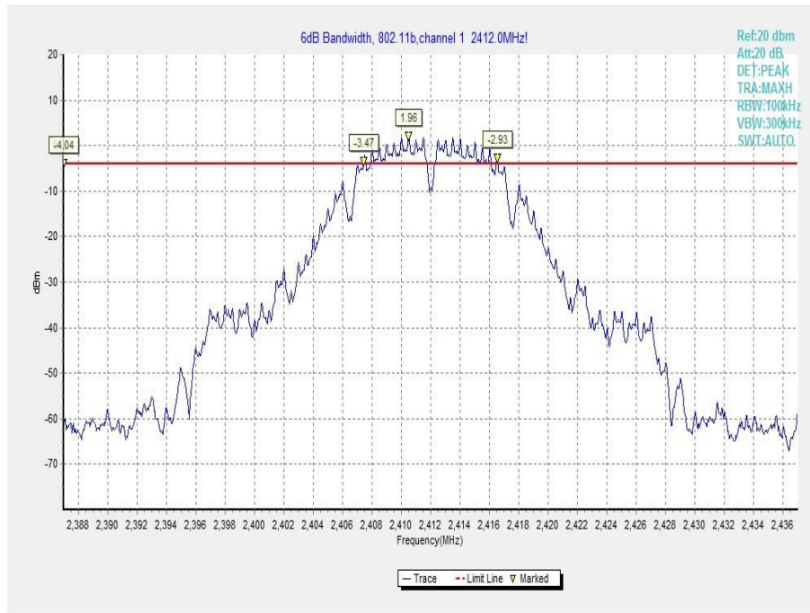
Fig.A.4.1 Occupied 6dB Bandwidth(802.11b,Ch 1)
