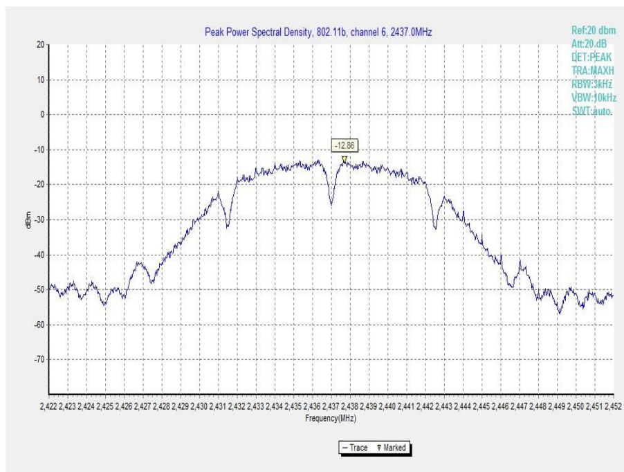
Fig.A.3.2 Power Spectral Density (802.11b, Ch 6)
