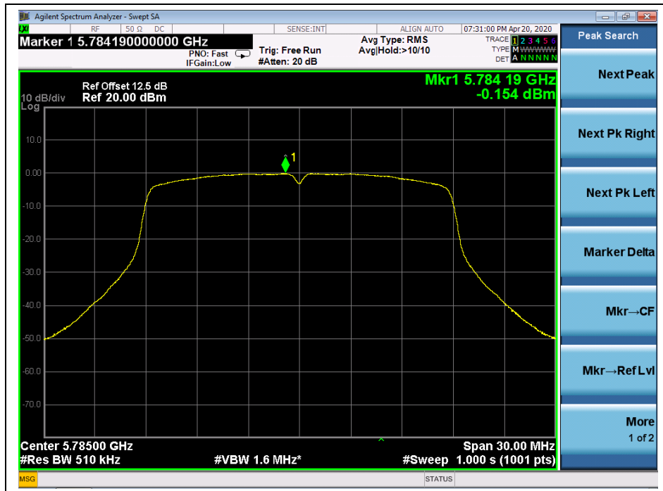
(Channel 157,5785MHz, 802.11ac (VHT20), ANT 0)
