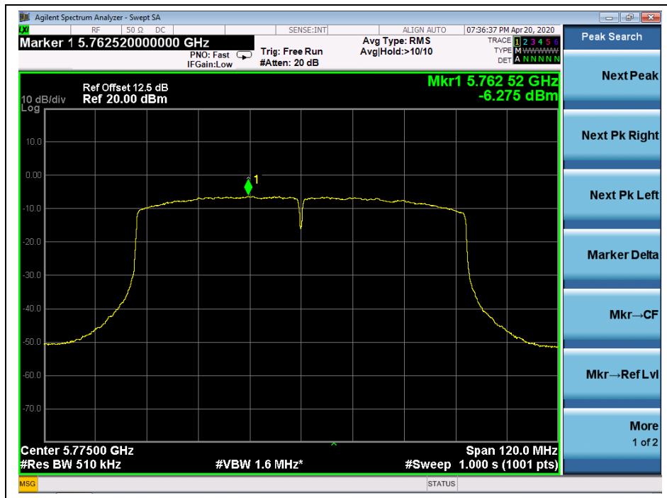
(Channel 155,5775MHz, 802.11ac(VHT80), ANT 0)
