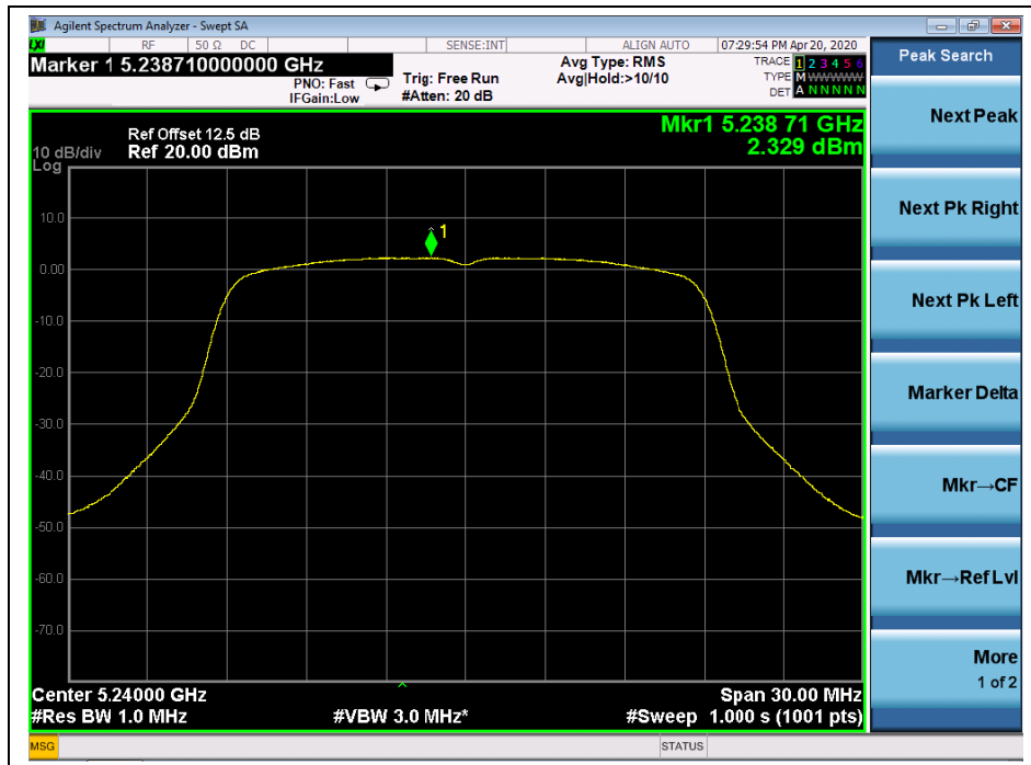
(Channel 48, 5240MHz, 802.11ac (VHT20), ANT 0)
