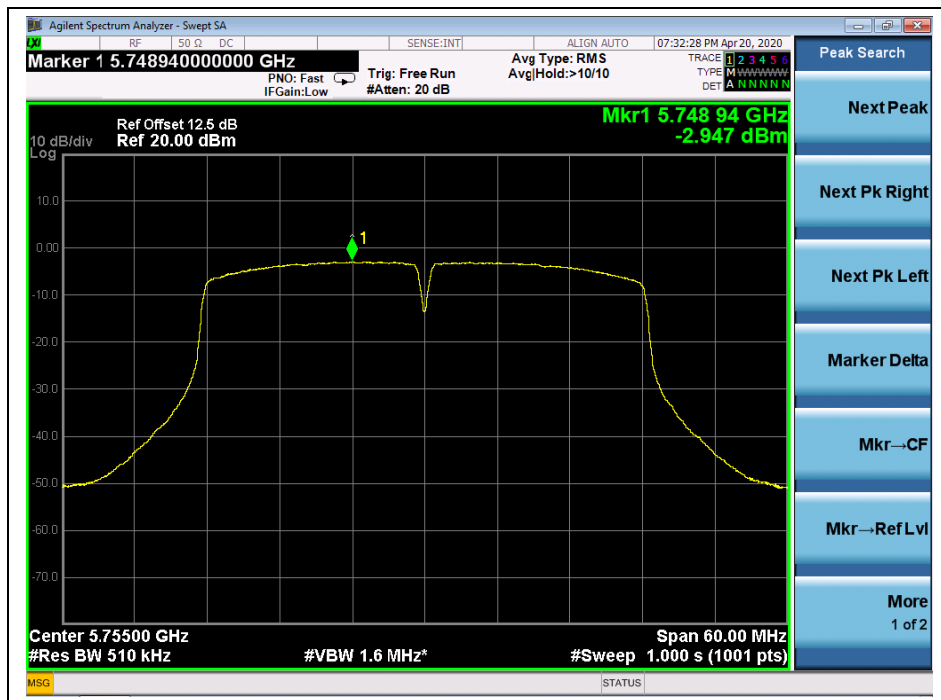
(Channel 151, 5755MHz, 802.11ac (VHT40), ANT 0)
