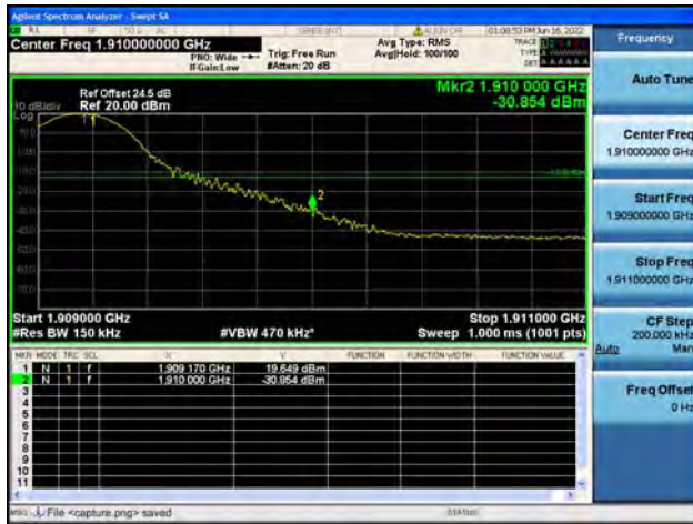
B2 / 15MHz / High CH / QPSK / 1 RB
