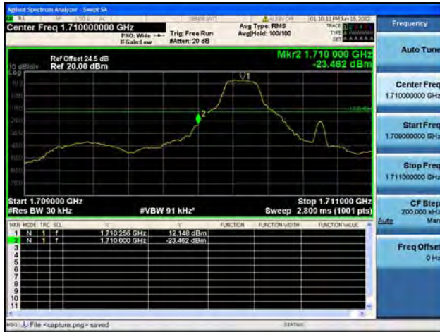
B4 / 1.4MHz / High CH / QPSK / 1 RB
