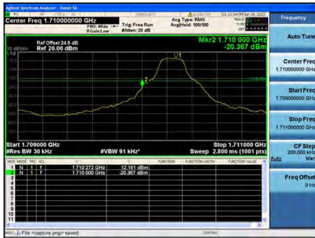
B4 / 3MHz / High CH / QPSK / 1 RB
