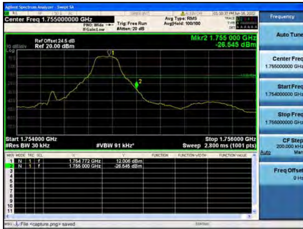
B4 / 1.4MHz / High CH / QPSK / 1 RB
