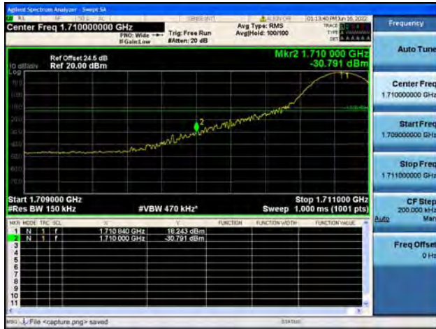
B4 / 15MHz / High CH / QPSK / 1 RB
