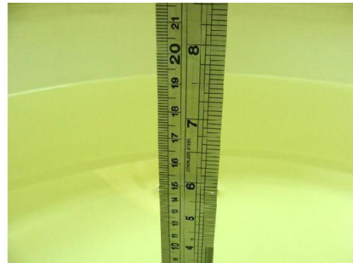
Fig 7.2 Photo of Liquid Height for Body SAR
