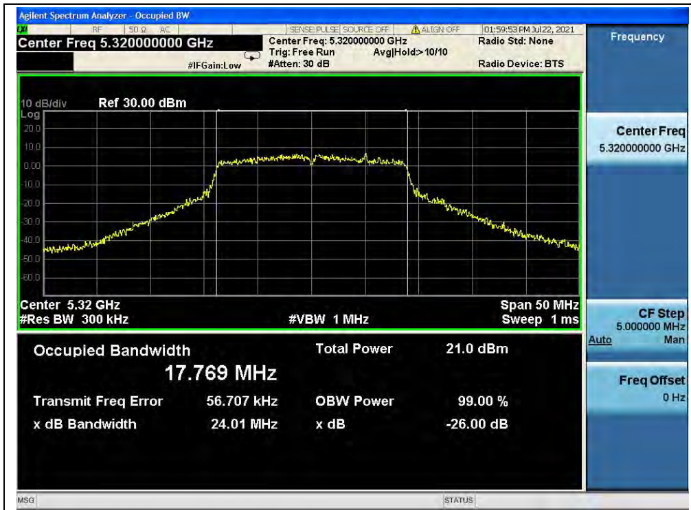
(Channel 64, 5320MHz, 802.11ac (VHT20))
