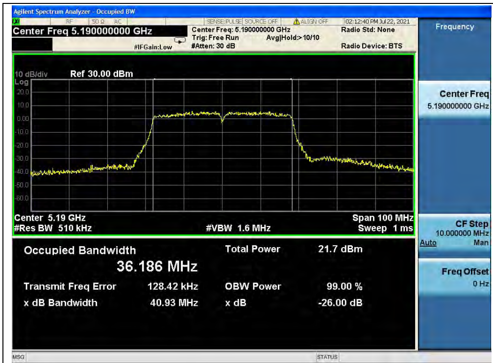
(Channel 38, 5190MHz, 802.11ac (VHT40))
