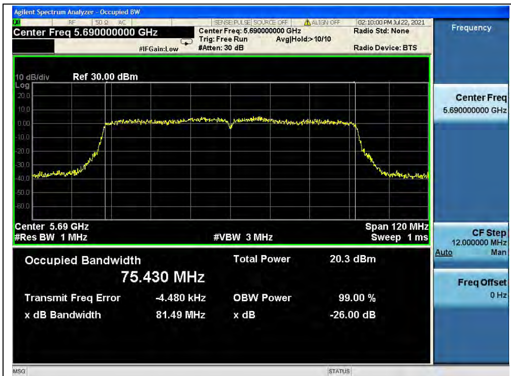
(Channel 138, 5690MHz, 802.11ac (VHT80))
