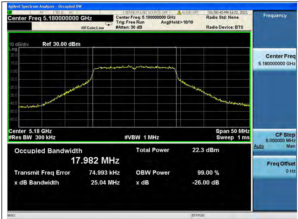
(Channel 36, 5180MHz, 802.11ac (VHT20))
