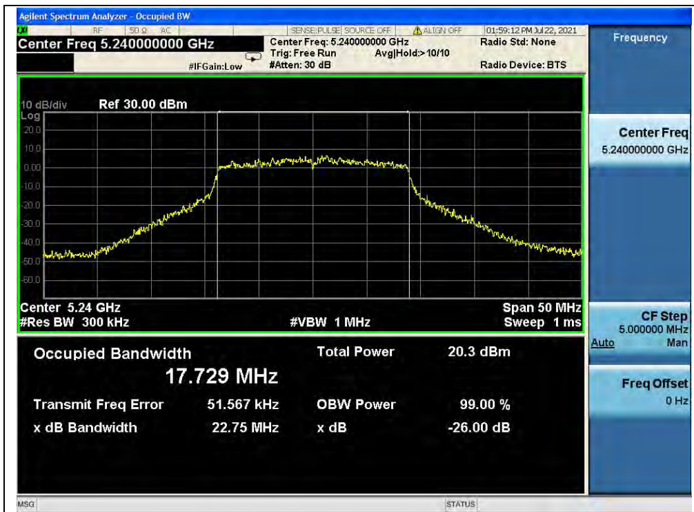
(Channel 48, 5240MHz, 802.11ac (VHT20))
