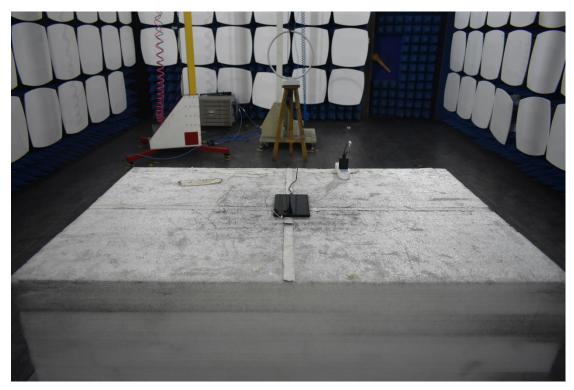
3. Radiated emission (9KHz-30MHz)
