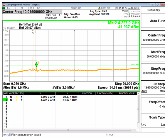
n48 (30MHz-20GHz) 40M DFT-s-OFDM QPSK Inner_1RB_Right High
