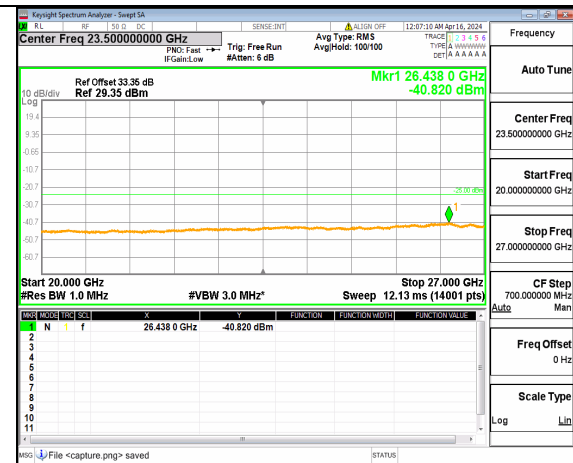
n41 (20GHz-27GHz) 100M DFT-s-OFDM QPSK Inner_1RB_Left High
