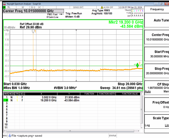
n48 (30MHz-20GHz) 20M DFT-s-OFDM BPSK Inner_1RB_Left Low
