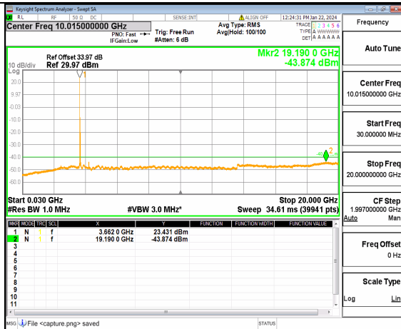
n48 (30MHz-20GHz) 40M DFT-s-OFDM QPSK Inner_1RB_Left High
