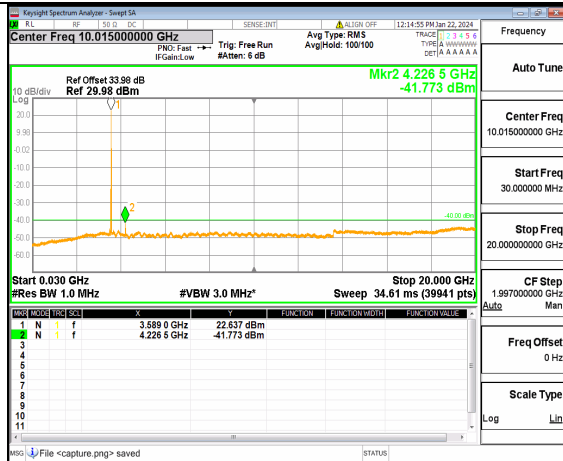
n48 (30MHz-20GHz) 40M DFT-s-OFDM QPSK Inner_1RB_Right Low
