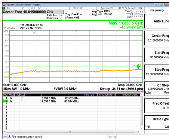
n48 (30MHz-20GHz) 20M DFT-s-OFDM QPSK Inner_1RB_Right High
