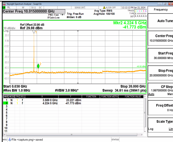
n48 (30MHz-20GHz) 40M DFT-s-OFDM BPSK Inner_1RB_Right Low
