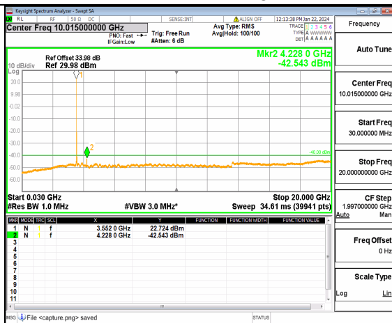
n48 (30MHz-20GHz) 40M DFT-s-OFDM QPSK Inner_1RB_Left Low
