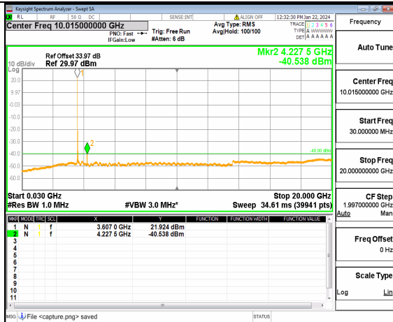
n48 (30MHz-20GHz) 40M DFT-s-OFDM QPSK Inner_1RB_Left Mid
