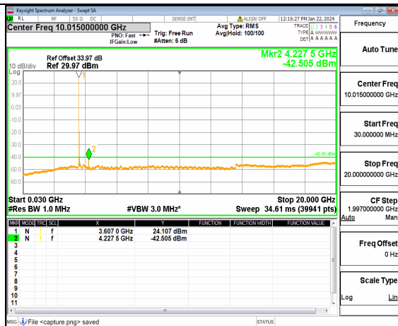
n48 (30MHz-20GHz) 40M DFT-s-OFDM BPSK Inner_1RB_Left Mid
