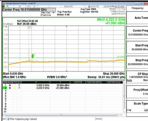
n48 (30MHz-20GHz) 40M DFT-s-OFDM BPSK Inner_1RB_Left Low
