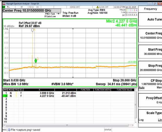
n48 (30MHz-20GHz) 40M DFT-s-OFDM BPSK Inner_1RB_Right High
