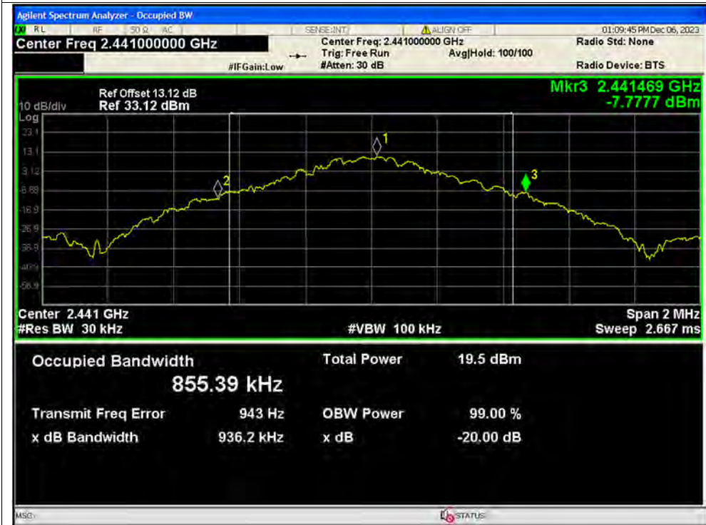
-20dB Bandwidth NVNT 1-DH5 2441MHz Ant1
