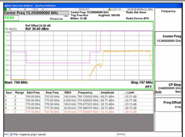
B13 / 10MHz / Low CH / QPSK / FULL RB
