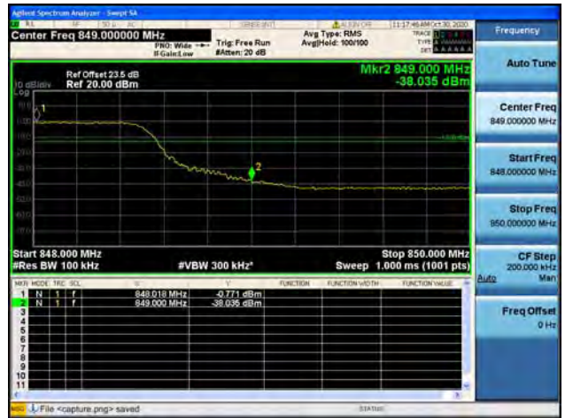
Band5 / 10MHz / High CH / QPSK / FULL RB
