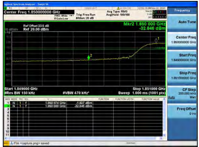
Band2 / 15MHz / High CH / QPSK / FULL RB
