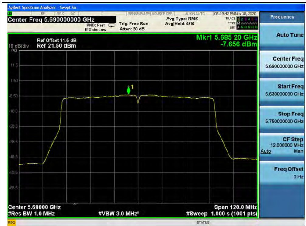
(Channel 138, 5690MHz, 802.11ac (VHT80), ANT1)
