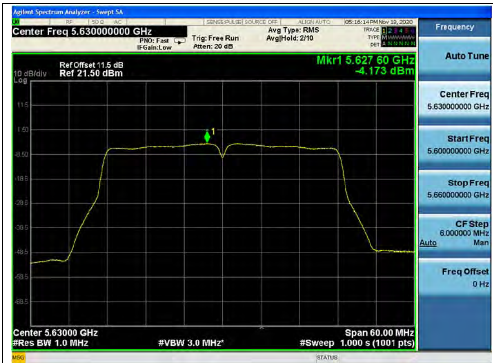
(Channel 126, 5630MHz, 802.11ac (VHT40), ANT1)
