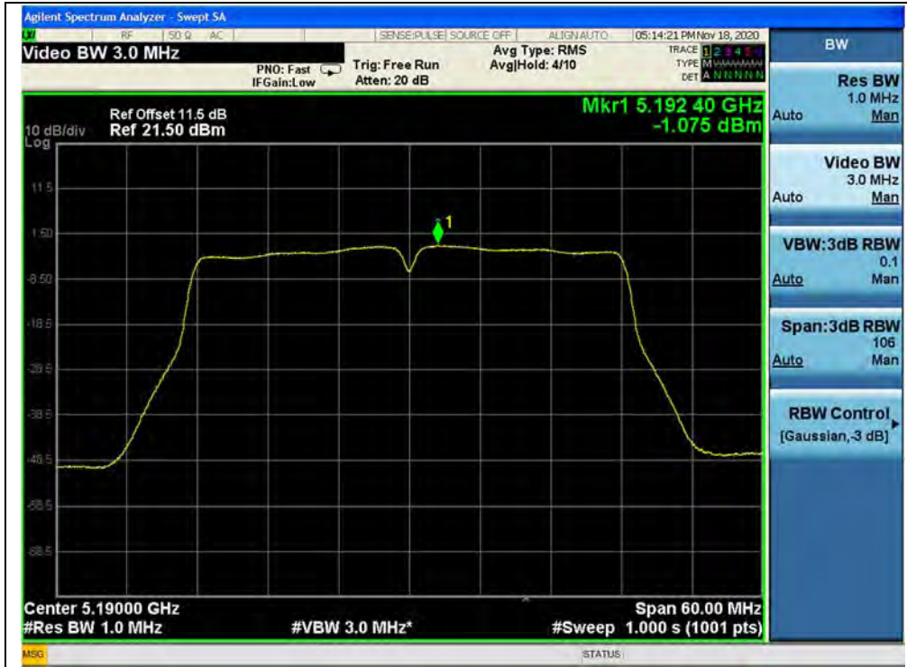
(Channel 38, 5190MHz, 802.11ac (VHT40), ANT1)
