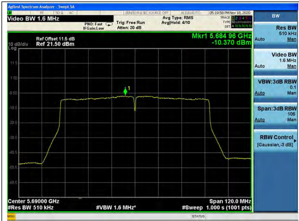
(Channel 138, 5690MHz, 802.11ac (VHT80), ANT1)
