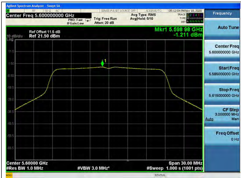
(Channel 120, 5600MHz, 802.11ac (VHT20), ANT1)
