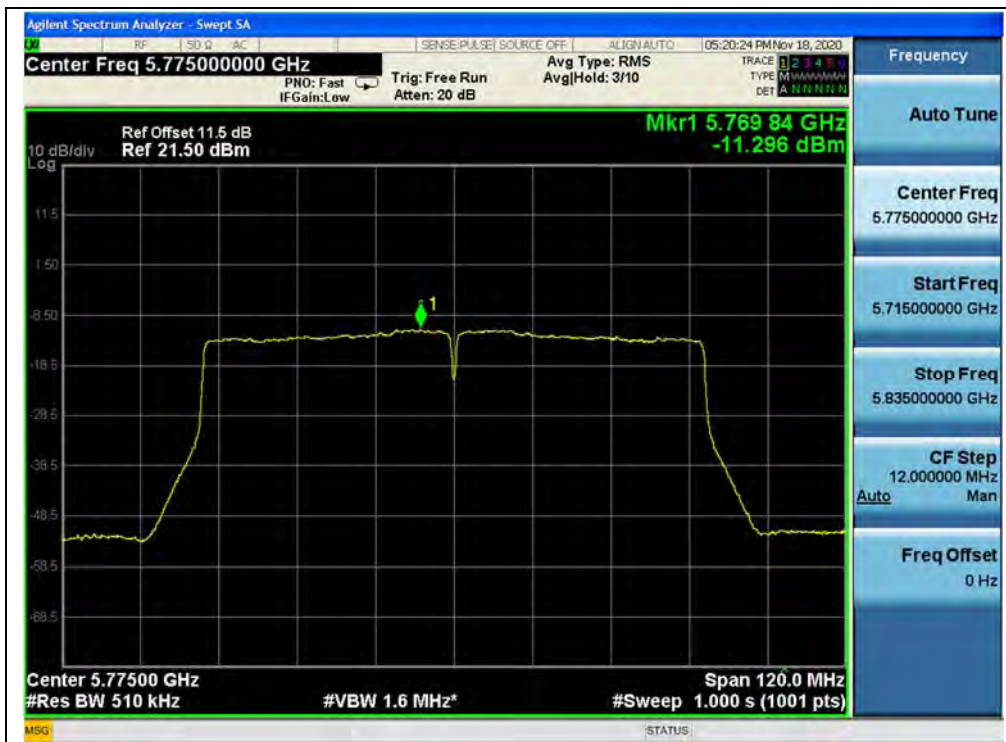
(Channel 155, 5775MHz, 802.11ac (VHT80), ANT1)
