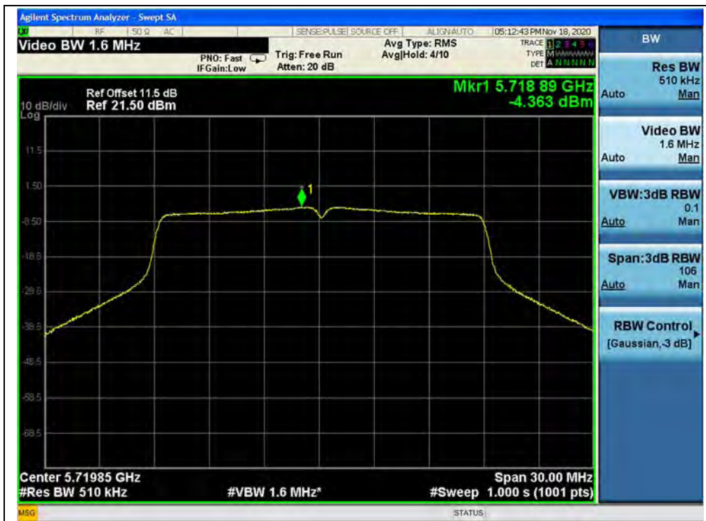
(Channel 144, 5720MHz, 802.11ac(VHT20), ANT1)
