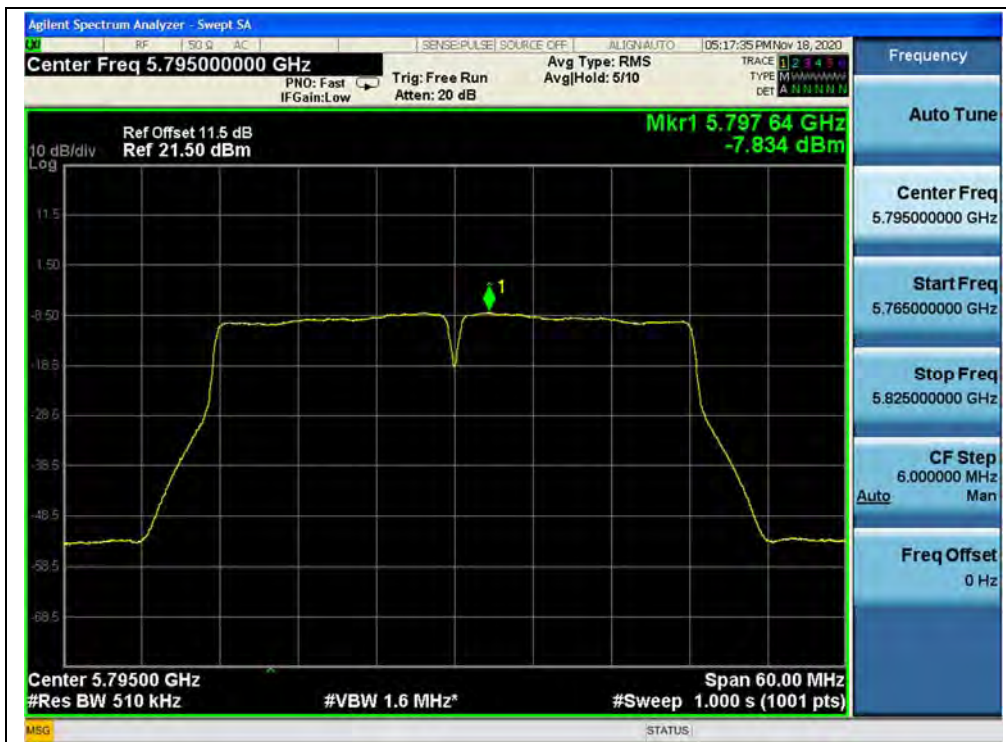
(Channel 159, 5795MHz, 802.11ac (VHT40), ANT1)
