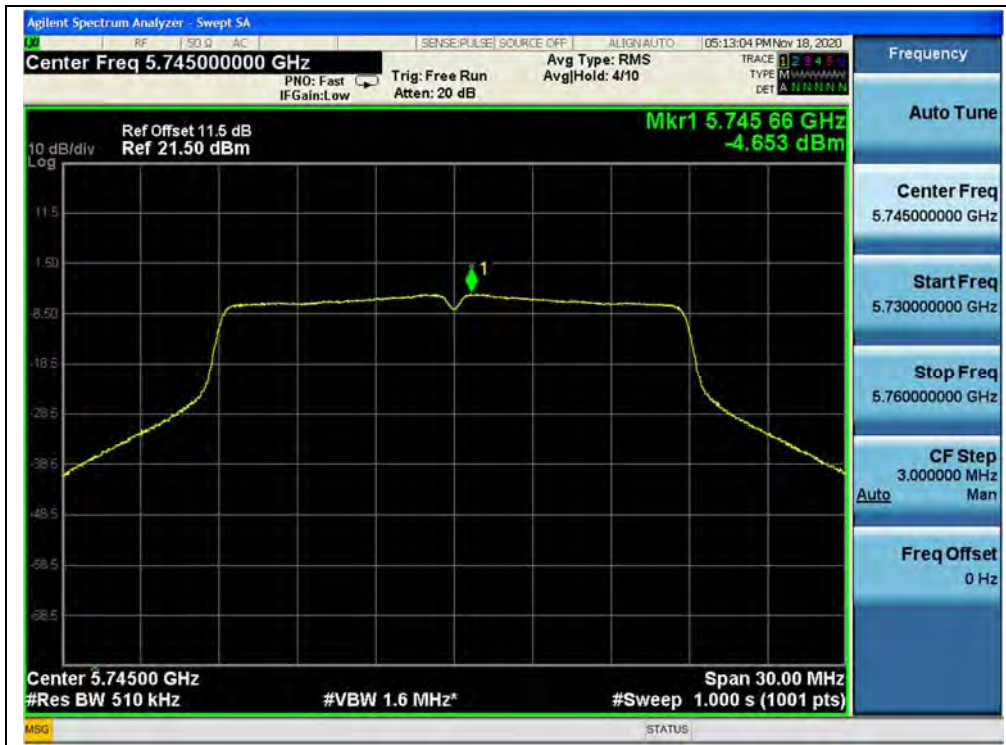
(Channel 149, 5745MHz, 802.11ac (VHT20), ANT1)
