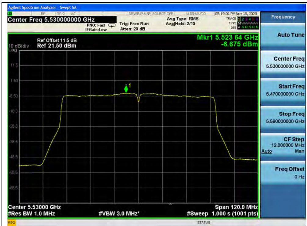
(Channel 106, 5530MHz, 802.11ac (VHT80), ANT1)
