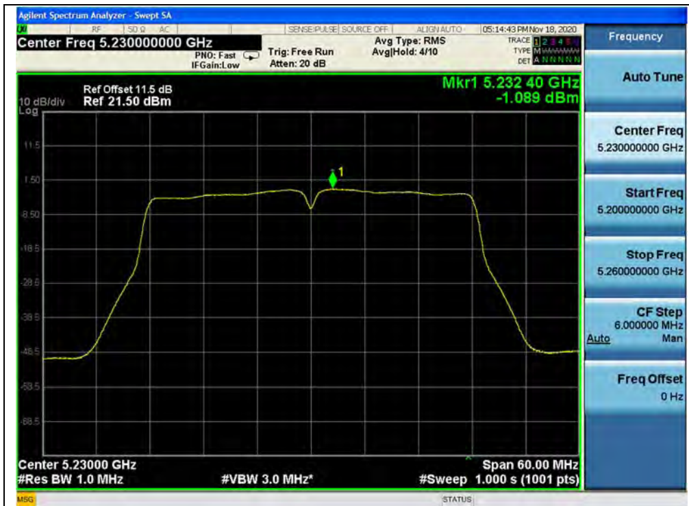
(Channel 46, 5230MHz, 802.11ac (VHT40), ANT1)
