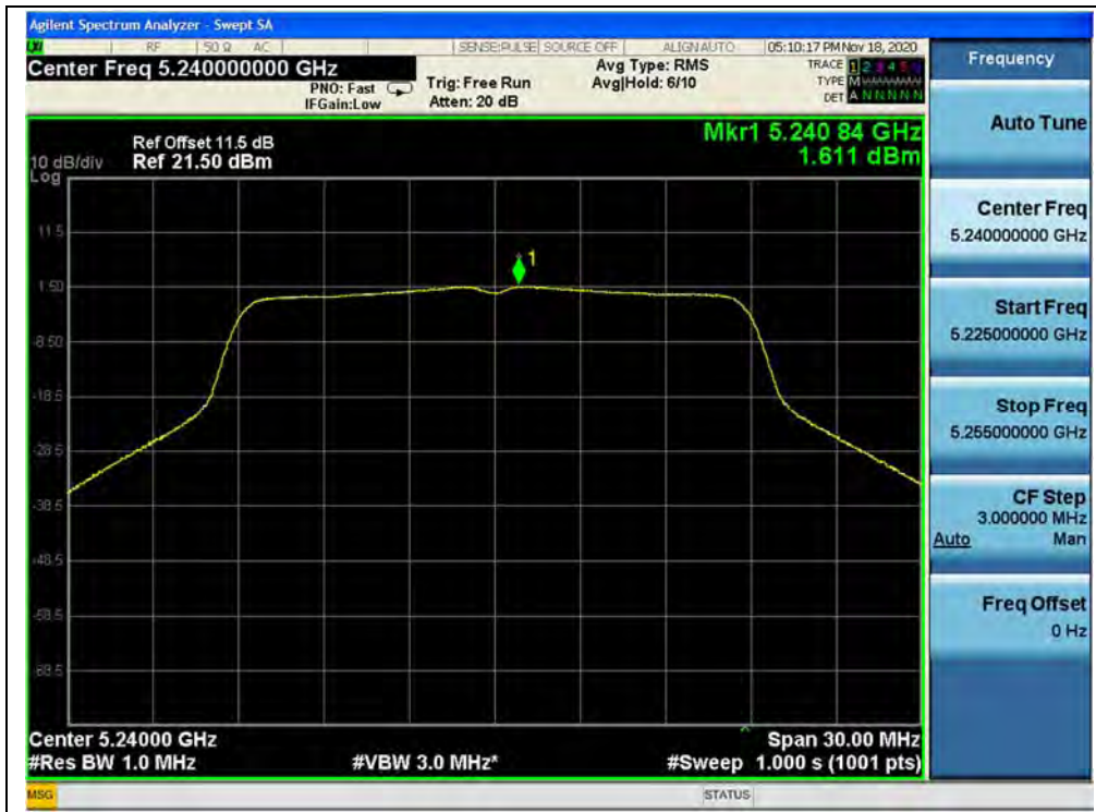
(Channel 48, 5240MHz, 802.11ac (VHT20), ANT1)
