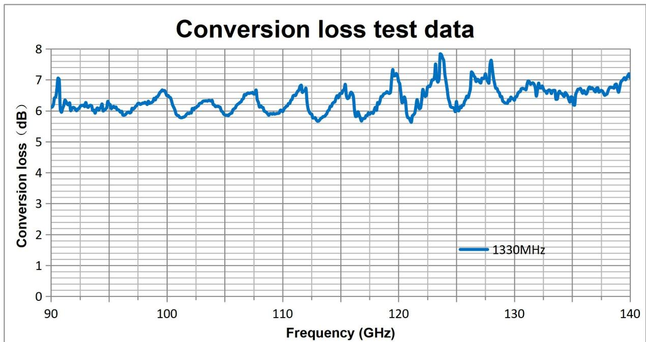
针对 RS FSW 系列, 中频 1330MHz, RF = -20 dBm, L.O. = (RF-/+IF)/9@7dBm, Bias = 0 mA
