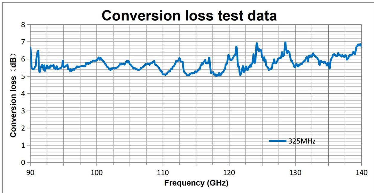
针对 KEYSIGHT N90x0B 系列, 中频 325MHz, RF= -20 dBm, L.O. = (RF-/+IF)/18@7dBm, Bias = 0 mA
