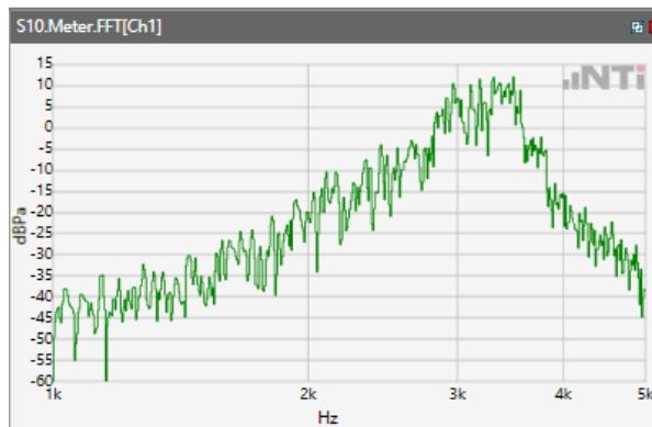
Distortion (Noise) RCV (packed): 36.2 dB
