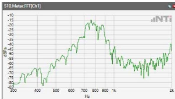
Distortion (Noise) RCV (packed): 36.99 dB
