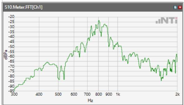
Distortion (Noise) RCV (packed): 34.85 dB
