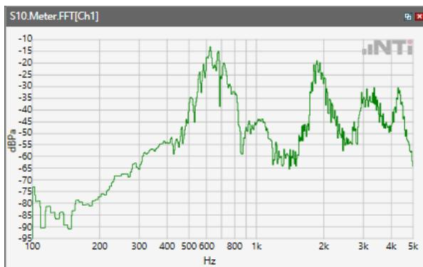
Distortion (Noise) RCV (packed): 37.72 dB
