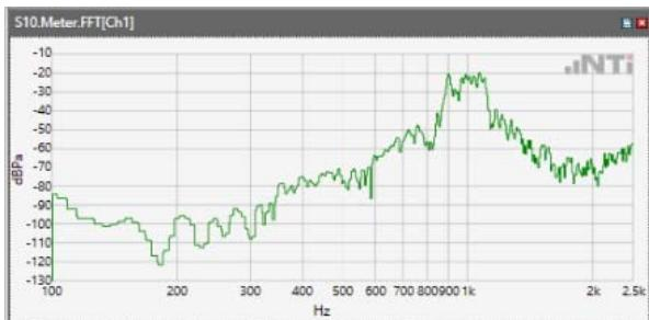
Distortion (Noise) RCV (packed): 32.77 dB
