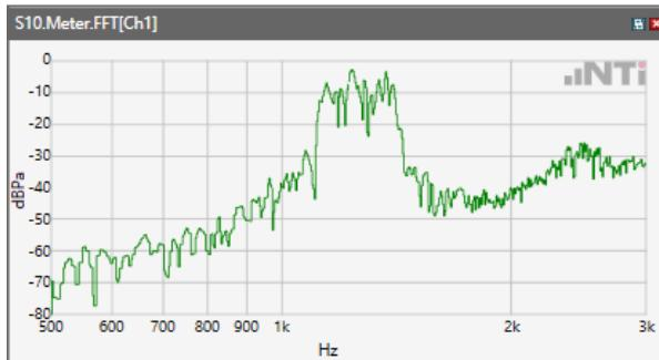
Distortion (Noise) RCV (packed): 40.63 dB
