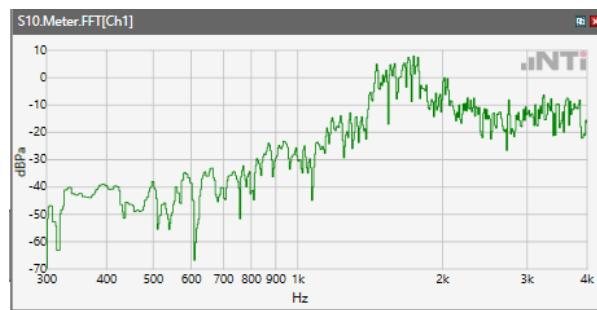
Distortion (Noise) RCV (packed): 38.62 dB
