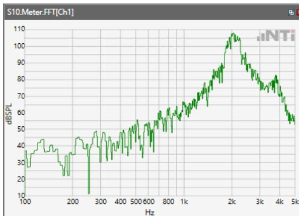
Distortion (Noise) RCV (packed): 46.1 dB
