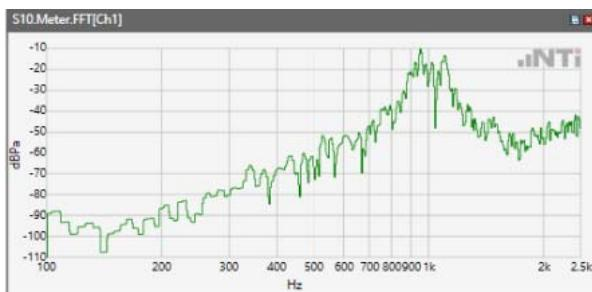
Distortion (Noise) RCV (packed): 39.95 dB
