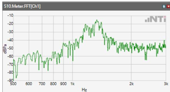
Distortion (Noise) RCV (packed): 35.05 dB
