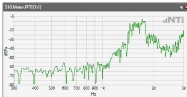
Distortion (Noise) RCV (packed): 37.49 dB
