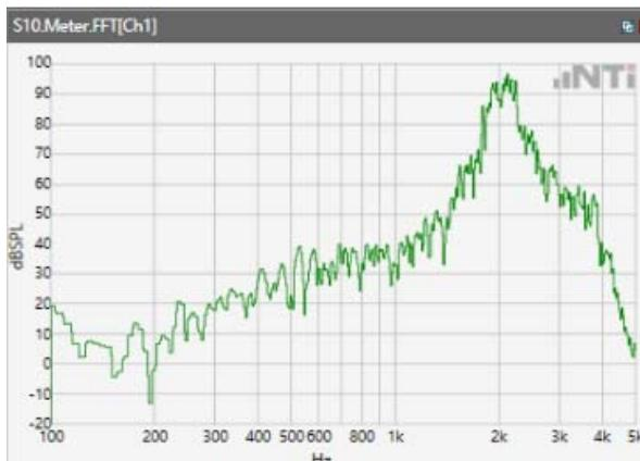
Distortion (Noise) RCV (packed): 44.33 dB
