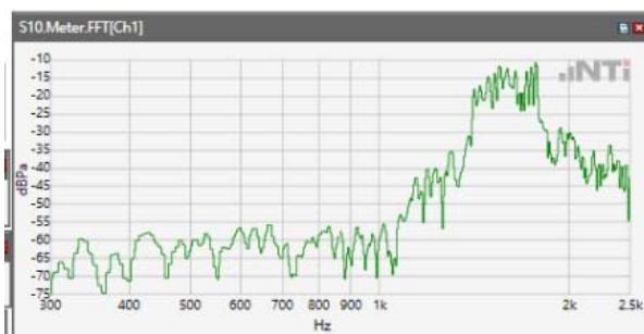
Distortion (Noise) RCV (packed): 38.48 dB
