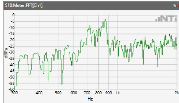
Distortion (Noise) RCV (packed): 41.28 dB
