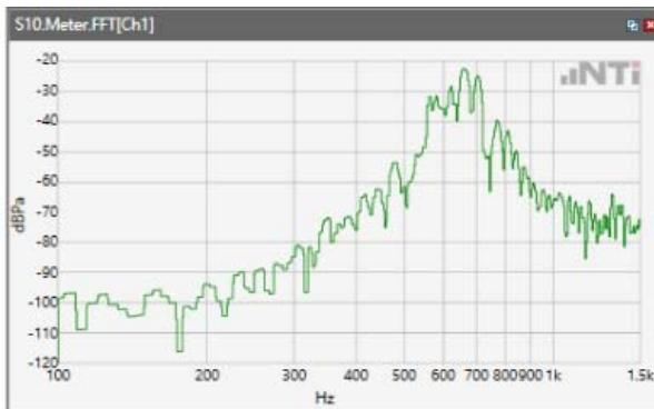
Distortion (Noise) RCV (packed): 30.71 dB
