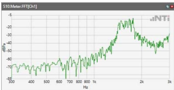
Distortion (Noise) RCV (packed): 32.6 dB
