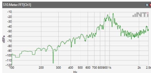
Distortion (Noise) RCV (packed): 38.32 dB
