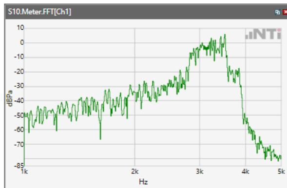
Distortion (Noise) RCV (packed): 36.85 dB
