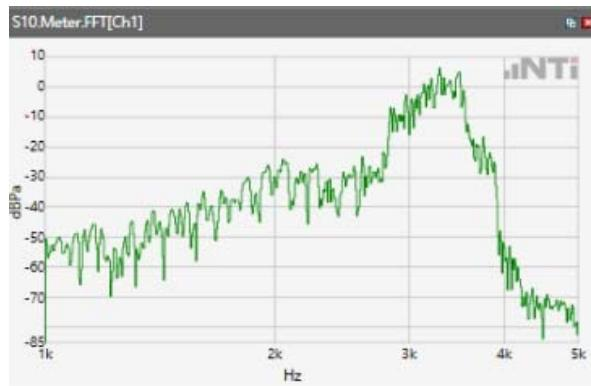
Distortion (Noise) RCV (packed): 37.77 dB
