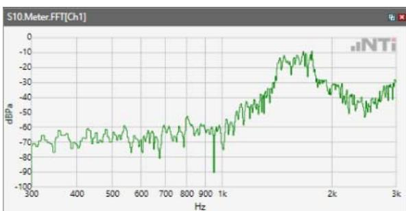
Distortion (Noise) RCV (packed): 35.49 dB
