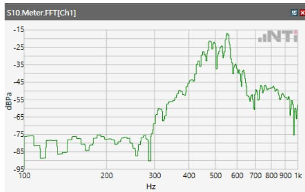
Distortion (Noise) RCV (packed): 38.83 dB
