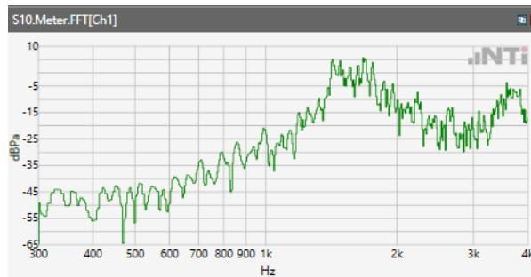
Distortion (Noise) RCV (packed): 38.22 dB
