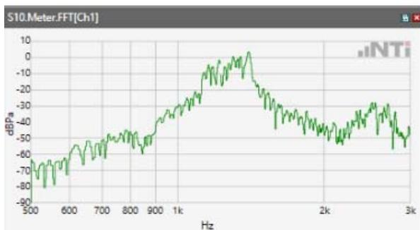
Distortion (Noise) RCV (packed): 42.19 dB
