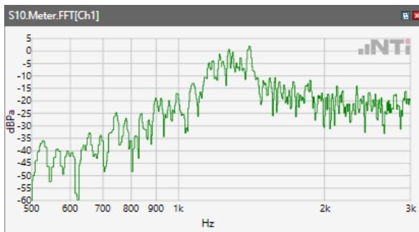
Distortion (Noise) RCV (packed): 38.04 dB
