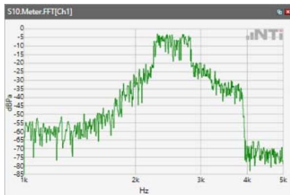
Distortion (Noise) RCV (packed): 36.42 dB
