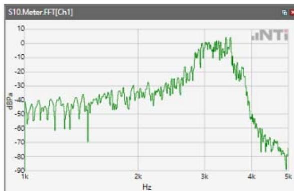
Distortion (Noise) RCV (packed): 33.1 dB
