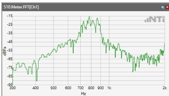
Distortion (Noise) RCV (packed): 39.54 dB
