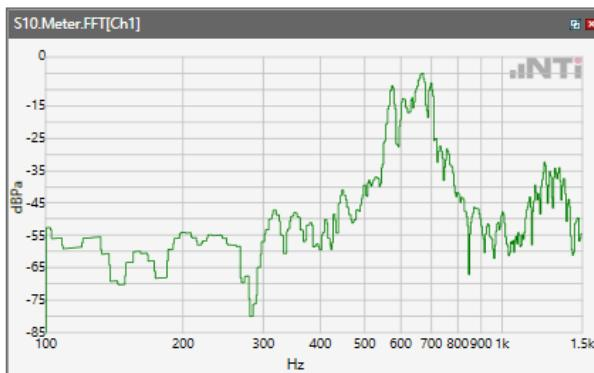
Distortion (Noise) RCV (packed): 45.41 dB
