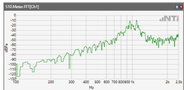
Distortion (Noise) RCV (packed): 41.17 dB
