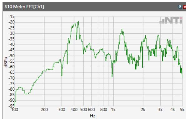
Distortion (Noise) RCV (packed): 40.43 dB
