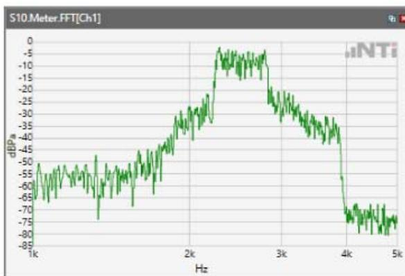
Distortion (Noise) RCV (packed): 36.85 dB
