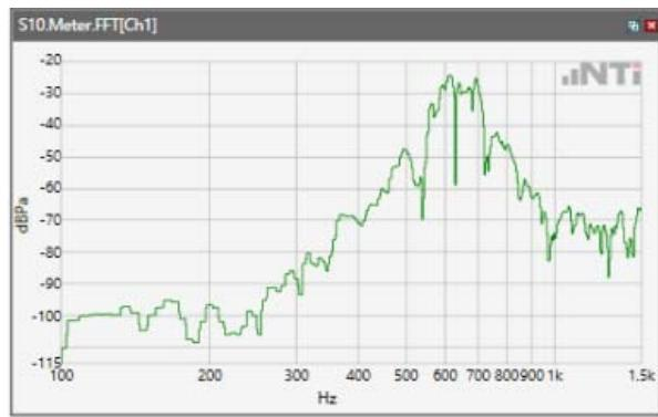
Distortion (Noise) RCV (packed): 38.92 dB
