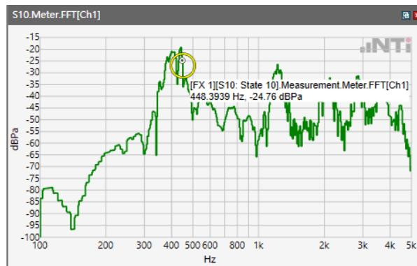
Distortion (Noise) RCV (packed): 40.14 dB
