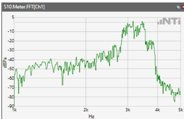
Distortion (Noise) RCV (packed): 38.63 dB
