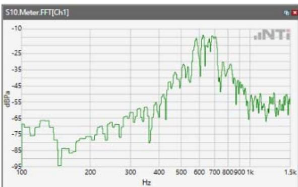
Distortion (Noise) RCV (packed): 36.61 dB
