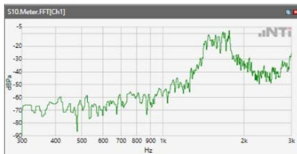
Distortion (Noise) RCV (packed): 34.49 dB
