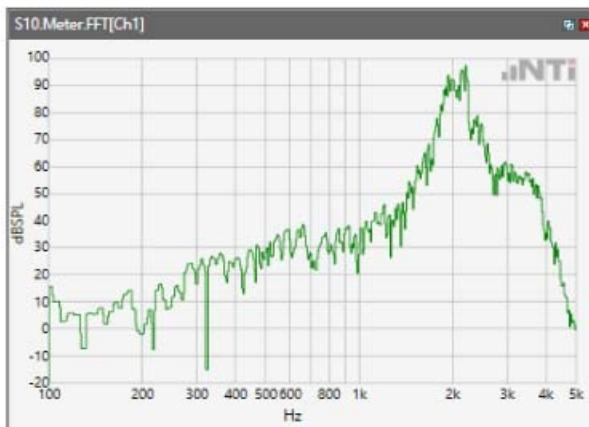
Distortion (Noise) RCV (packed): 45.47 dB
