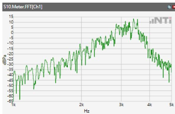
Distortion (Noise) RCV (packed): 36.96 dB
