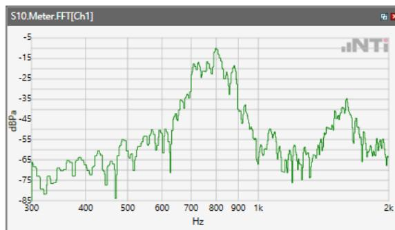
Distortion (Noise) RCV (packed): 43.98 dB
