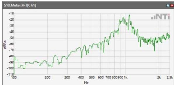
Distortion (Noise) RCV (packed): 41.18 dB
