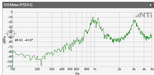
Distortion (Noise) RCV (packed): 37.84 dB
