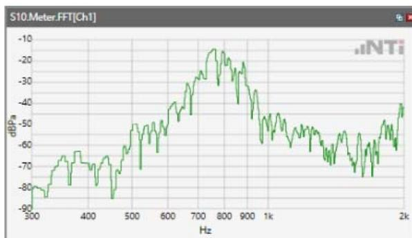
Distortion (Noise) RCV (packed): 37.17 dB
