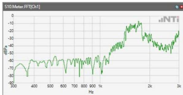
Distortion (Noise) RCV (packed): 37.39 dB
