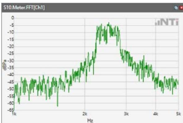
Distortion (Noise) RCV (packed): 46.14 dB
