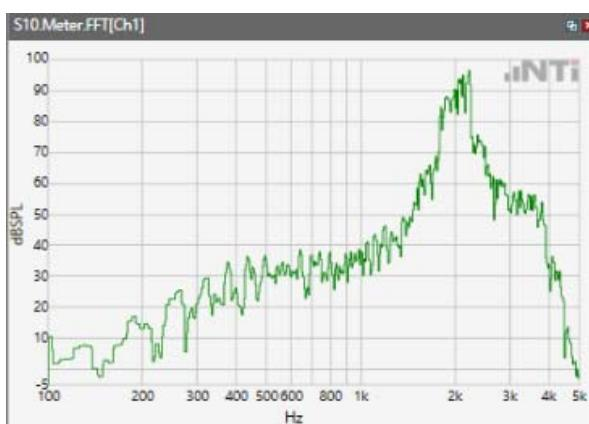
Distortion (Noise) RCV (packed): 44.91 dB
