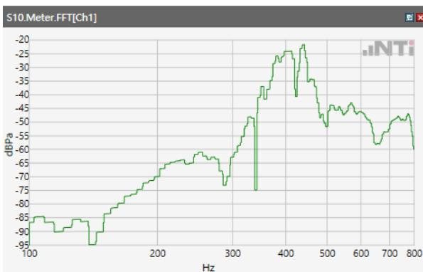
Distortion (Noise) RCV (packed): 39.65 dB
