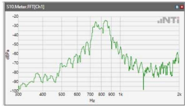
Distortion (Noise) RCV (packed): 34.2 dB
