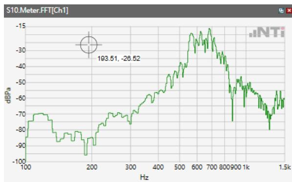
Distortion (Noise) RCV (packed): 38.08 dB
