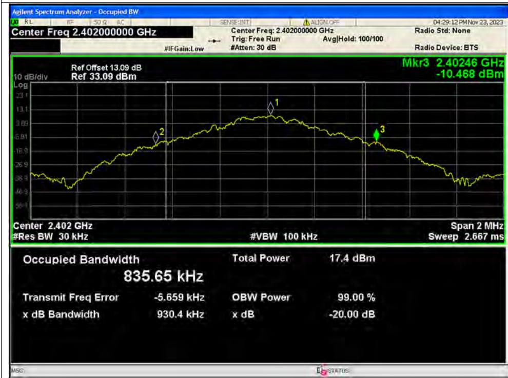
-20dB Bandwidth NVNT 1-DH5 2441MHz Ant1
