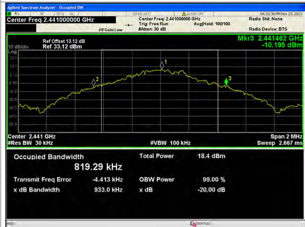
-20dB Bandwidth NVNT 1-DH5 2441MHz Ant1
