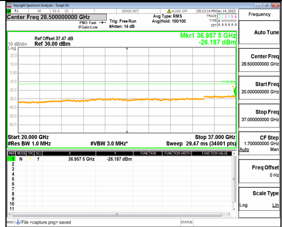
2A_n77(3450-3650MHz) (20GHz-37GHz) 30M DFT-s-OFDM BPSK Inner_1RB_Right High
