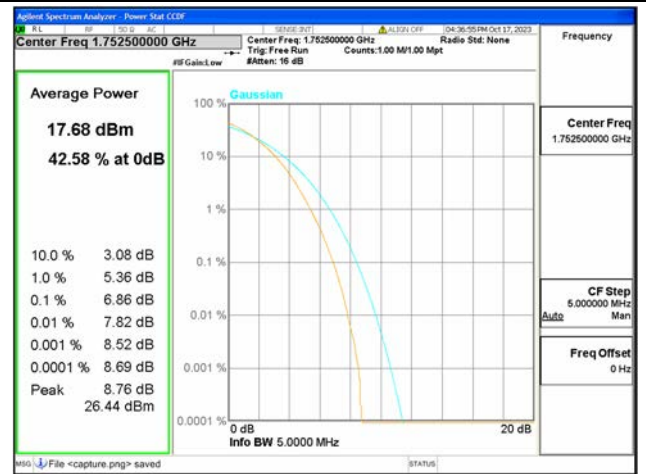
B4 / 5MHz / High CH / 256QAM
