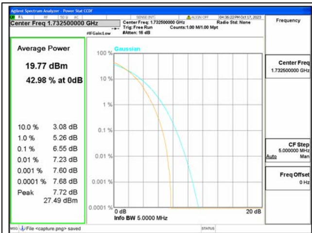
B4 / 5MHz / Mid CH / 64QAM
