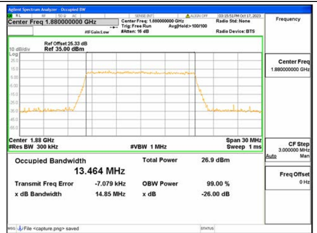
B2 / 15MHz / 256QAM/ Mid CH
