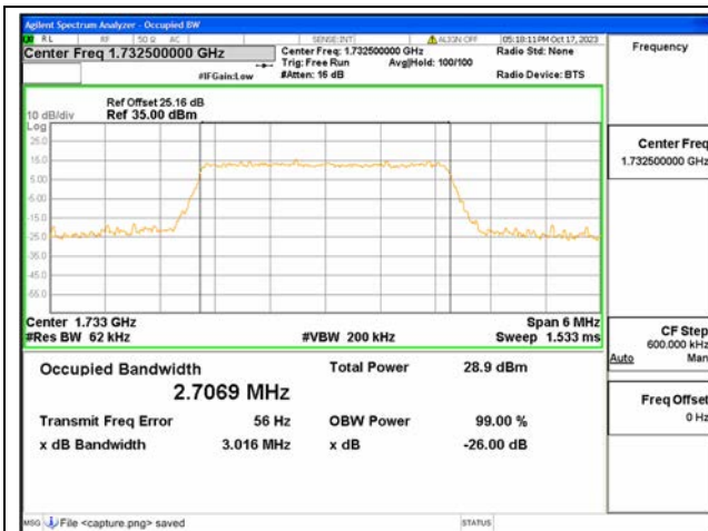
B4 / 3MHz / 64QAM/ Mid CH
