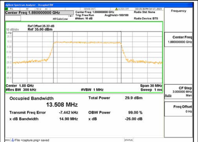
B2 / 15MHz / 16QAM/ Mid CH
