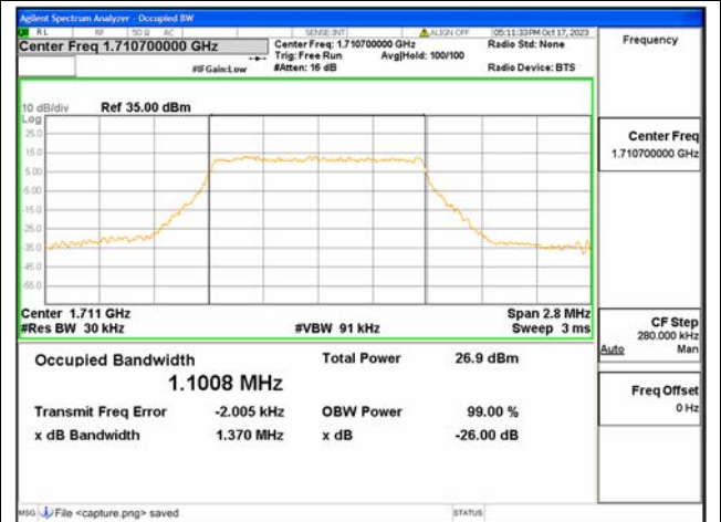
B4 / 1.4MHz / 256QAM/ Low CH
