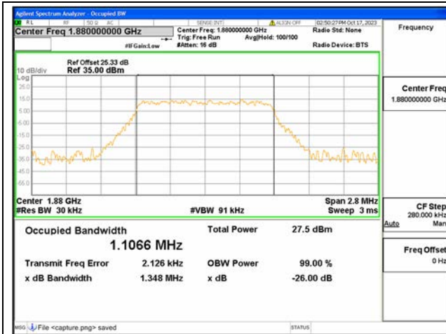
B2 / 1.4MHz / 64QAM/ Mid CH
