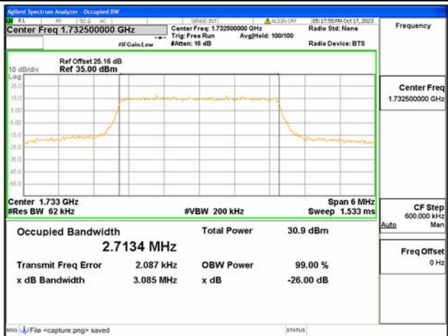
B4 / 3MHz / QPSK/ Mid CH
