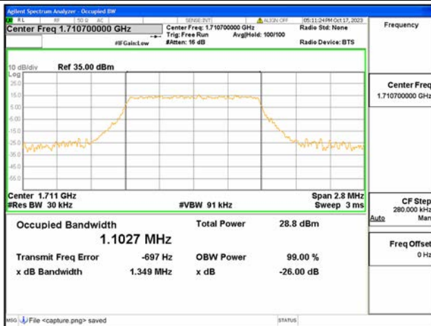
B4 / 1.4MHz / 64QAM/ Low CH
