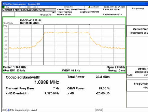
B2 / 1.4MHz / QPSK/ High CH
