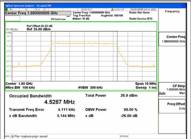
B2 / 5MHz / 256QAM/ Mid CH
