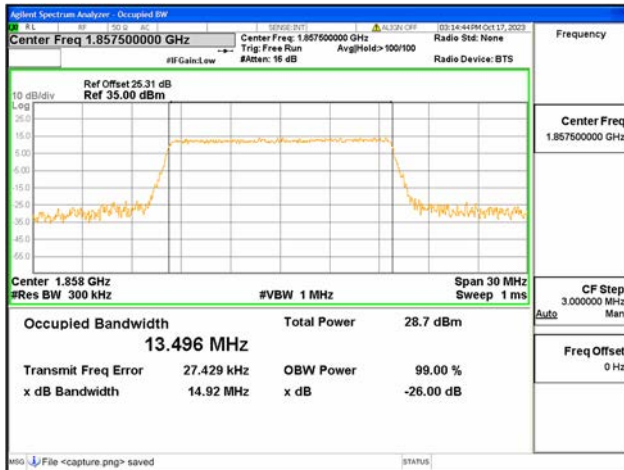
B2 / 15MHz / 64QAM/ Low CH
