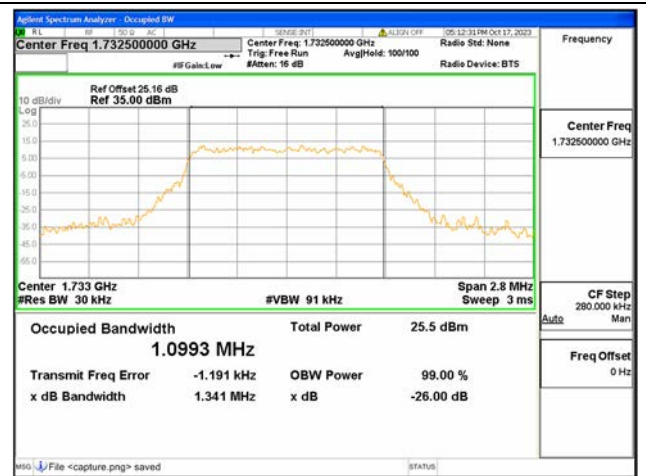
B4 / 1.4MHz / 256QAM/ Mid CH
