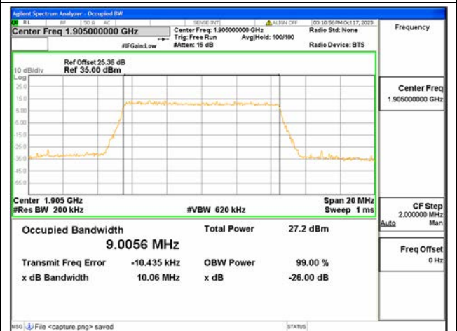
B2 / 10MHz / 256QAM/ High CH
