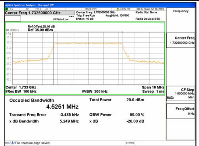
B4 / 5MHz / 16QAM/ Mid CH
