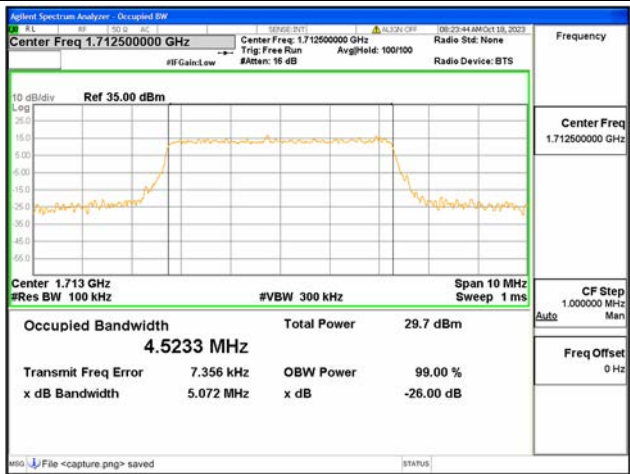
B4 / 5MHz / 64QAM/ Low CH
