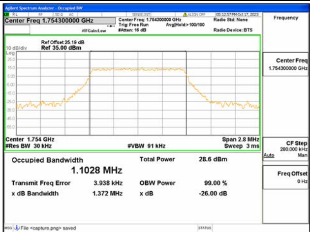
B4 / 1.4MHz / 64QAM/ High CH
