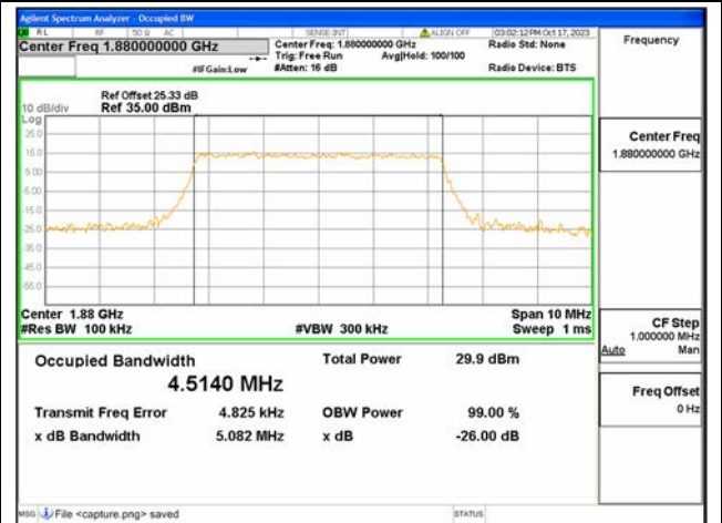
B2 / 5MHz / 16QAM/ Mid CH
