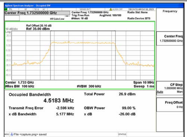
B4 / 5MHz / 256QAM/ Mid CH
