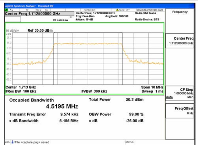
B4 / 5MHz / 16QAM/ Low CH
