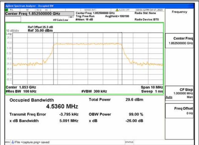
B2 / 5MHz / 16QAM/ Low CH
