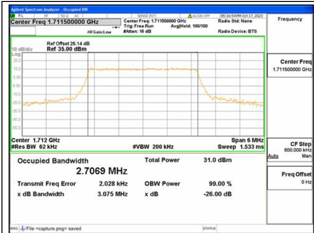
B4 / 3MHz / QPSK/ Low CH
