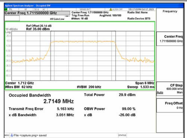
B4 / 3MHz / 16QAM/ Low CH
