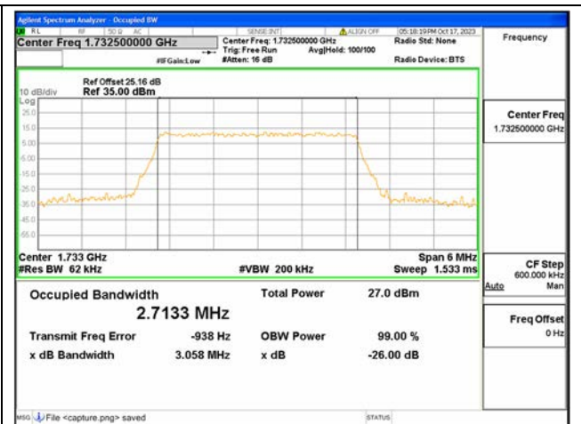
B4 / 3MHz / 256QAM/ Mid CH
