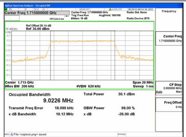
B4 / 10MHz / 16QAM/ Low CH
