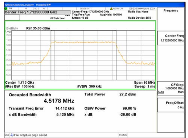
B4 / 5MHz / 256QAM/ Low CH
