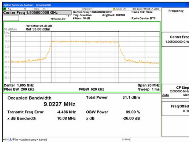
B2 / 10MHz / QPSK/ High CH
