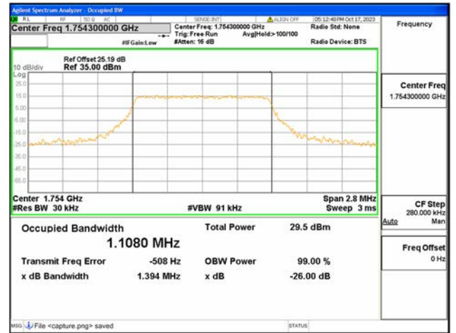
B4 / 1.4MHz / 16QAM/ High CH
