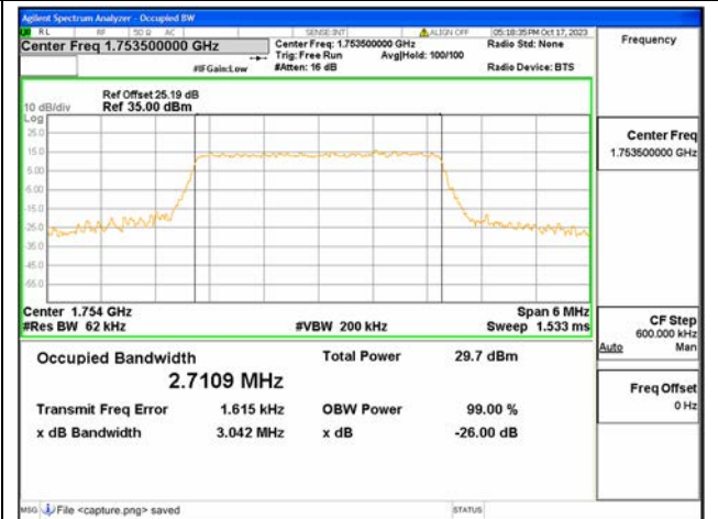
B4 / 3MHz / 16QAM/ High CH
