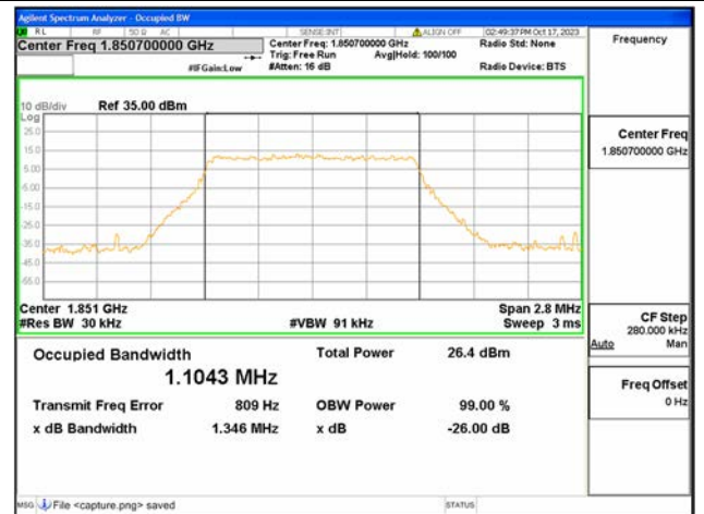
B2 / 1.4MHz / 256QAM/ Low CH
