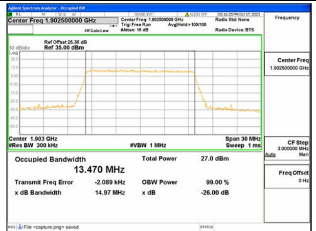
B2 / 15MHz / 256QAM/ High CH
