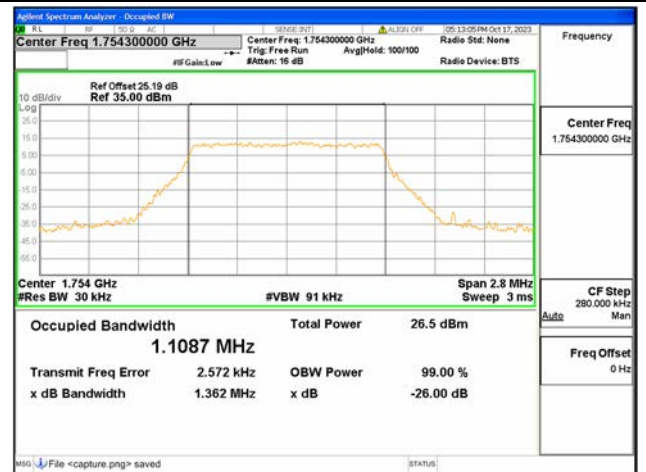
B4 / 1.4MHz / 256QAM/ High CH
