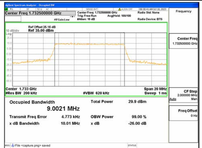
B4 / 10MHz / 16QAM/ Mid CH
