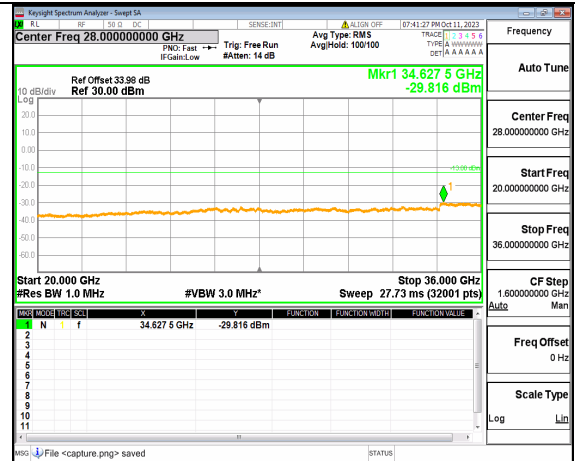
5A_n77(3450-3550MHz) (20GHz-36GHz) 30M DFT-s-OFDM QPSK Outer_Full High
