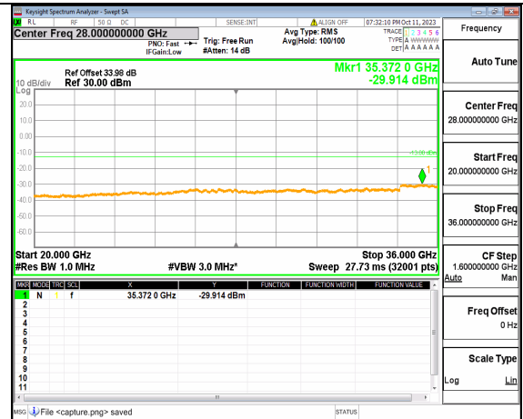
5A_n77(3450-3550MHz) (20GHz-36GHz) 30M DFT-s-OFDM BPSK Edge_1RB_Right Mid
