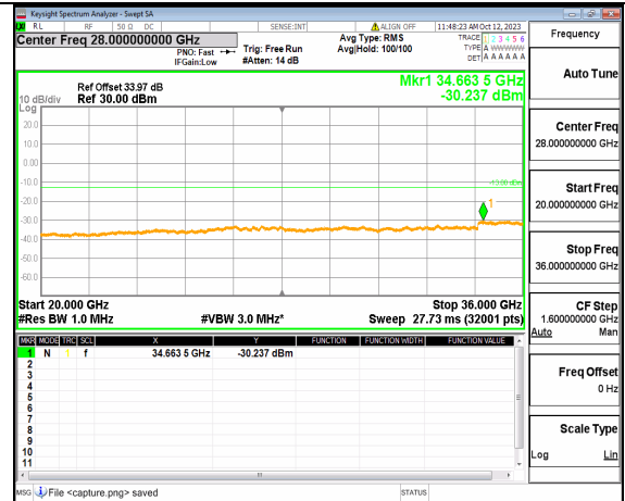
5A_n77(3450-3550MHz) (20GHz-36GHz) 60M DFT-s-OFDM QPSK Outer_Full Low
