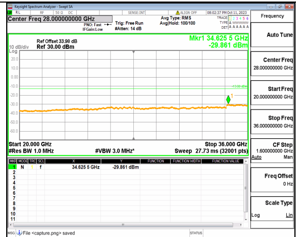
5A_n77(3450-3550MHz) (20GHz-36GHz) 40M DFT-s-OFDM BPSK Edge_1RB_Left High
