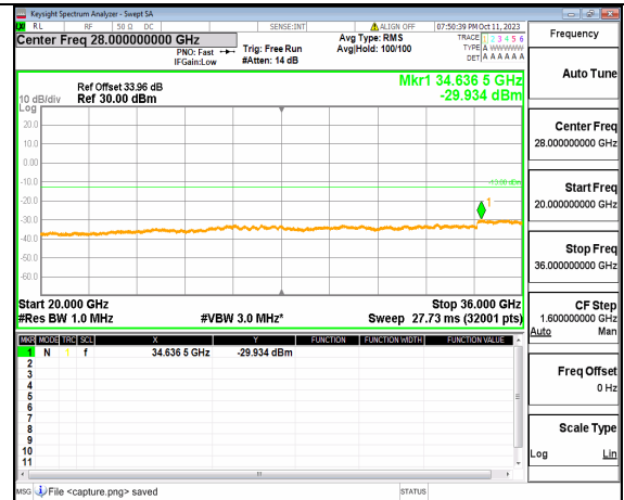
5A_n77(3450-3550MHz) (20GHz-36GHz) 40M DFT-s-OFDM QPSK Edge_1RB_Left Low
