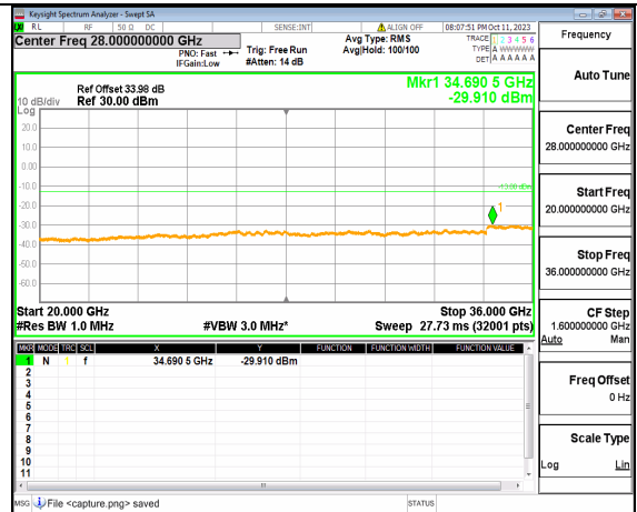
5A_n77(3450-3550MHz) (20GHz-36GHz) 40M DFT-s-OFDM QPSK Edge_1RB_Right High
