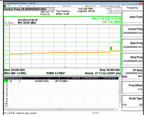
5A_n77(3450-3550MHz) (20GHz-36GHz) 40M DFT-s-OFDM BPSK Outer_Full Low
