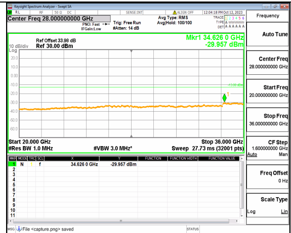
5A_n77(3450-3550MHz) (20GHz-36GHz) 60M DFT-s-OFDM QPSK Edge_1RB_Left High
