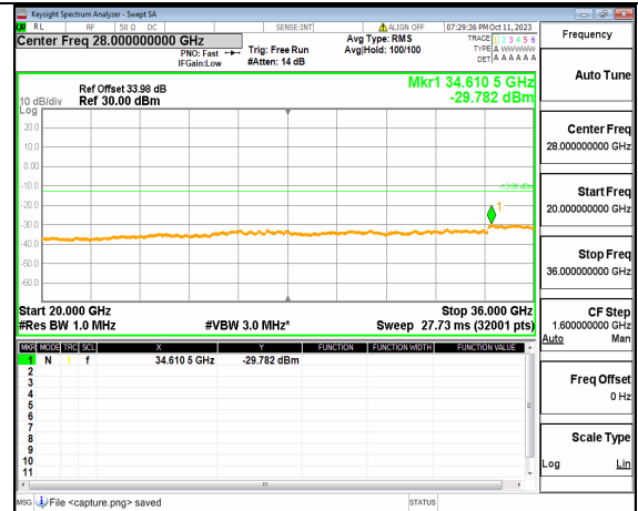
5A_n77(3450-3550MHz) (20GHz-36GHz) 30M DFT-s-OFDM BPSK Outer_Full Mid
