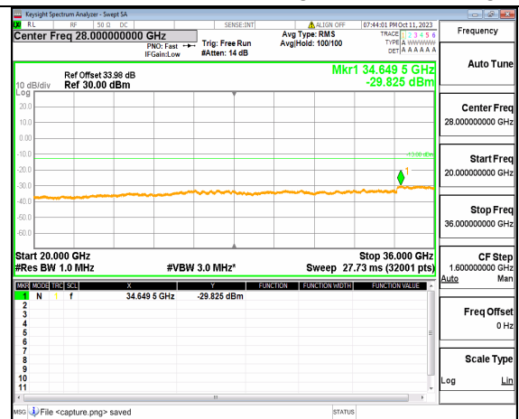
5A_n77(3450-3550MHz) (20GHz-36GHz) 30M DFT-s-OFDM QPSK Edge_1RB_Right High
