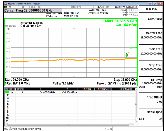
5A_n77(3450-3550MHz) (20GHz-36GHz) 60M DFT-s-OFDM QPSK Edge_1RB_Right Mid
