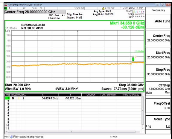
5A_n77(3450-3550MHz) (20GHz-36GHz) 50M DFT-s-OFDM QPSK Edge_1RB_Right High
