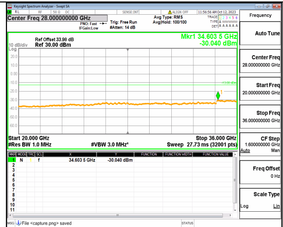
5A_n77(3450-3550MHz) (20GHz-36GHz) 60M DFT-s-OFDM QPSK Edge_1RB_Left Mid
