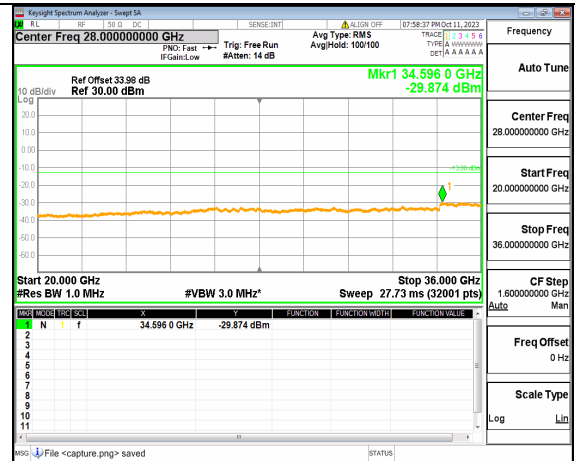
5A_n77(3450-3550MHz) (20GHz-36GHz) 40M DFT-s-OFDM QPSK Edge_1RB_Left Mid
