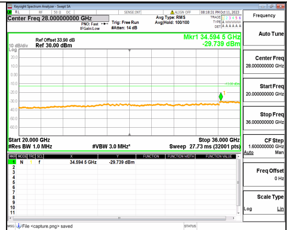
5A_n77(3450-3550MHz) (20GHz-36GHz) 50M DFT-s-OFDM BPSK Edge_1RB_Left Mid
