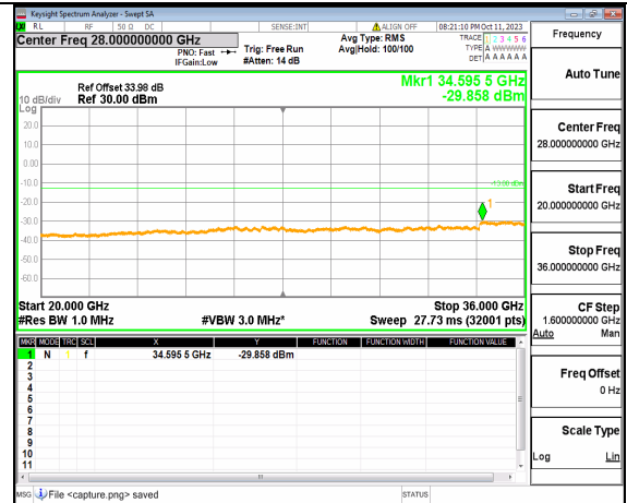
5A_n77(3450-3550MHz) (20GHz-36GHz) 50M DFT-s-OFDM QPSK Outer_Full Mid
