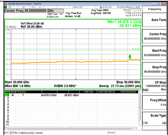
5A_n77(3450-3550MHz) (20GHz-36GHz) 30M DFT-s-OFDM QPSK Edge_1RB_Left Low
