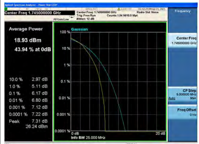
Band66 / 15MHz / Mid CH / 64QAM
