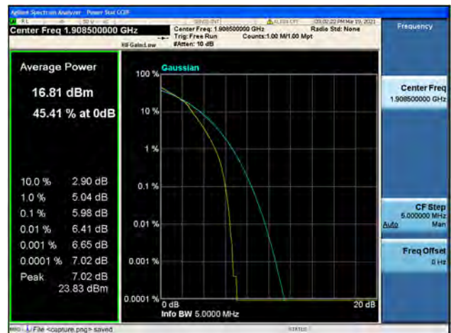
Band2 / 3MHz / High CH / 64QAM
