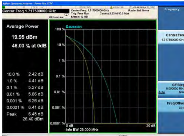
Band66 / 15MHz / Low CH / 64QAM
