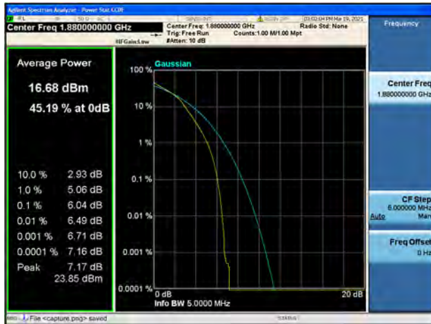
Band2 / 3MHz / High CH / 16QAM
