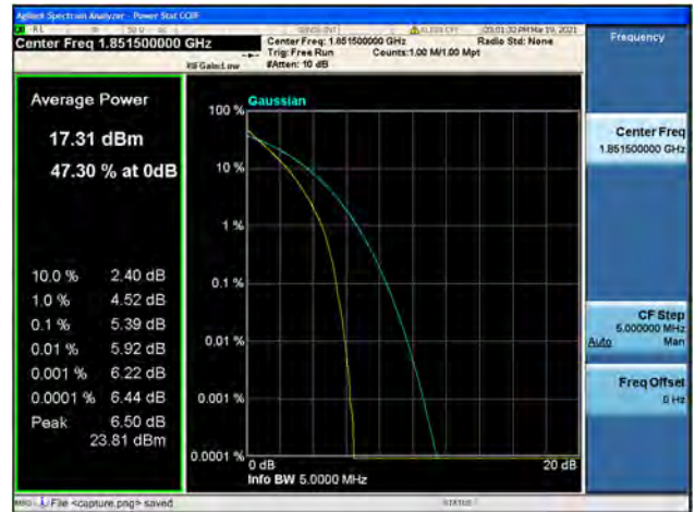
Band2 / 3MHz / Low CH / 64QAM
