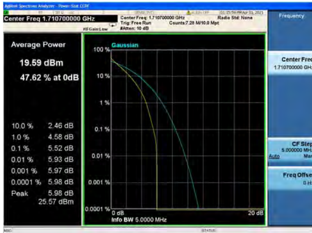
Band66 / 1.4MHz / Low CH / 64QAM
