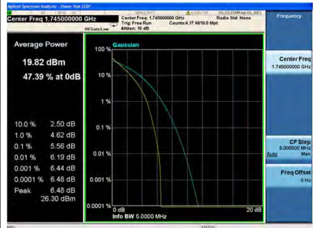
Band66 / 1.4MHz / Mid CH / 64QAM
