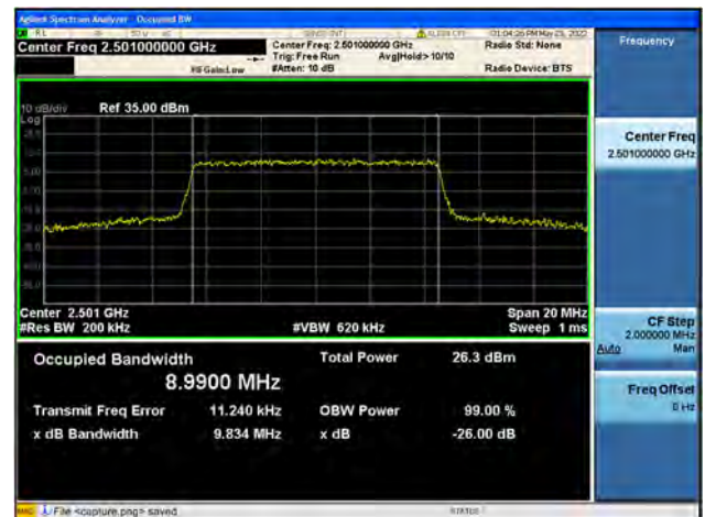
Band41 / 10MHz / Low CH / 64QAM
