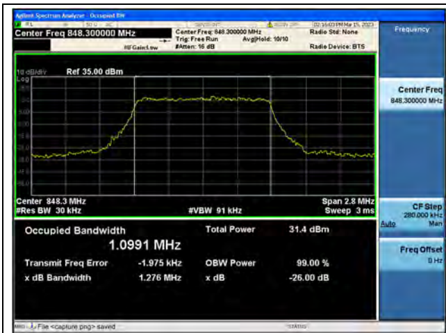
Band26 Part22 / 1.4MHz / QPSK/ High CH
