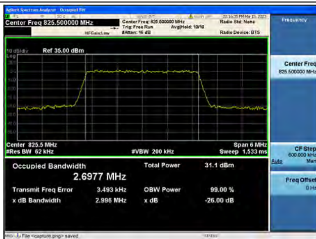
Band26 Part22 / 3MHz / 16QAM/ Low CH
