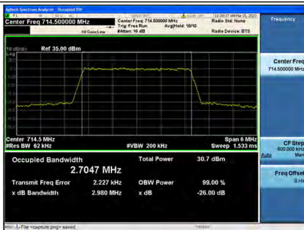
Band12 / 3MHz / 16QAM/ High CH
