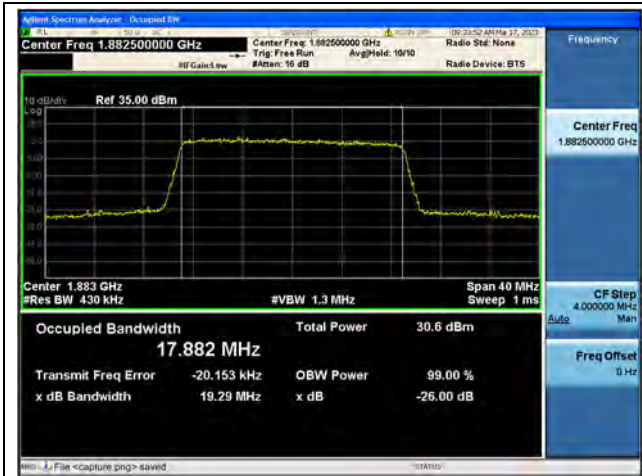
Band25 / 20MHz / QPSK/ Mid CH
