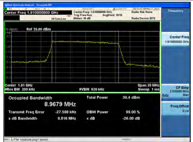
Band25 / 10MHz / QPSK/ High CH
