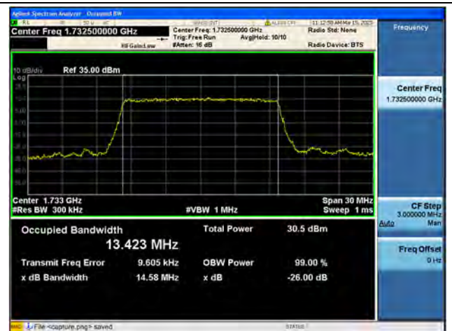
Band4 / 15MHz / 64QAM/ Mid CH
