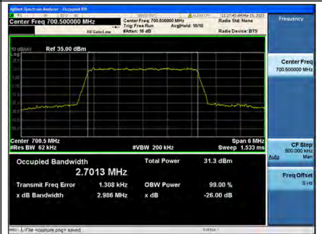
Band12 / 3MHz / QPSK/ Low CH
