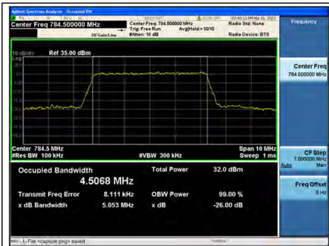
Band13 / 5MHz / QPSK/ High CH
