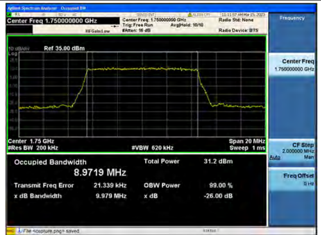
Band4 / 10MHz / QPSK/ High CH
