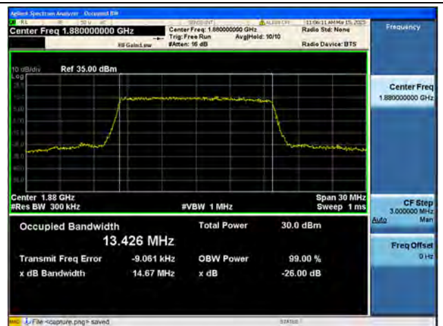
Band2 / 15MHz / 64QAM/ Mid CH
