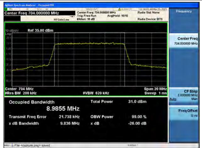
Band12 / 10MHz / QPSK/ Low CH
