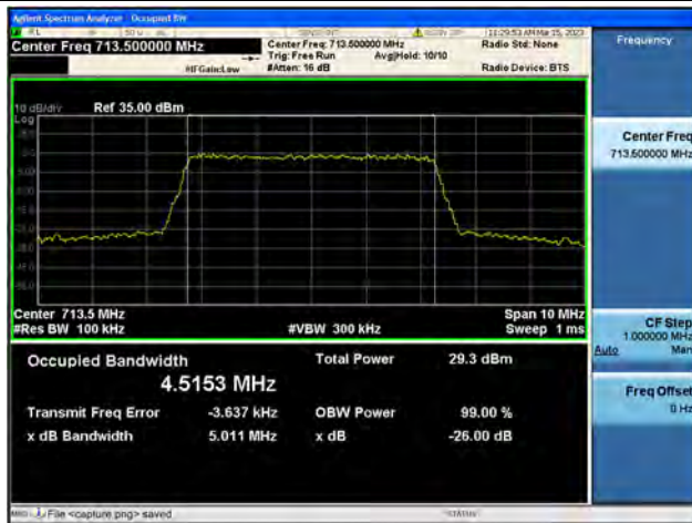
Band12 / 5MHz / 64QAM/ High CH
