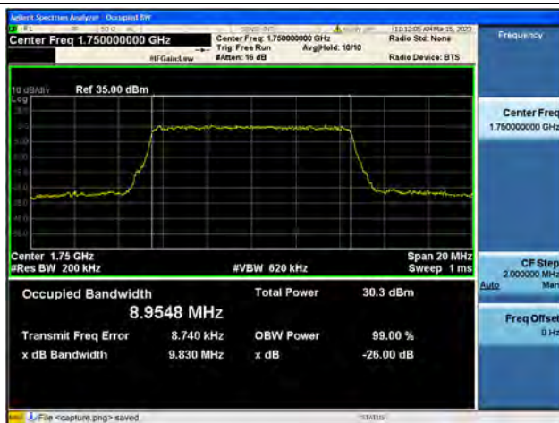
Band4 / 10MHz / 16QAM/ High CH
