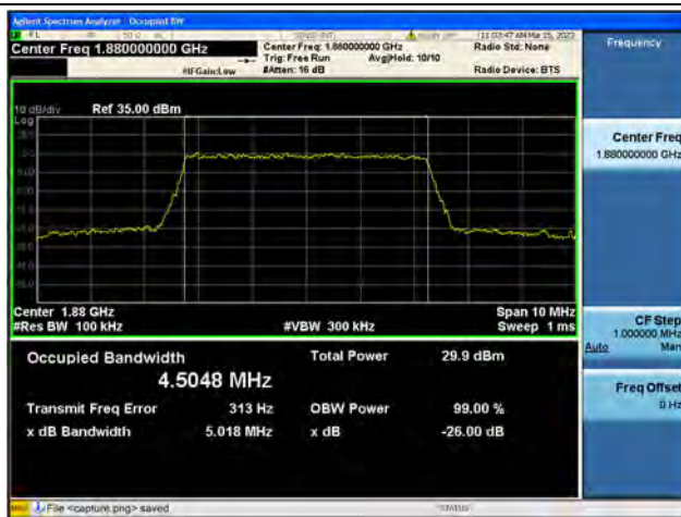
Band2 / 5MHz / 16QAM/ Mid CH
