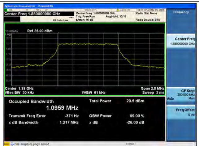
Band2 / 1.4MHz / 64QAM/ Mid CH
