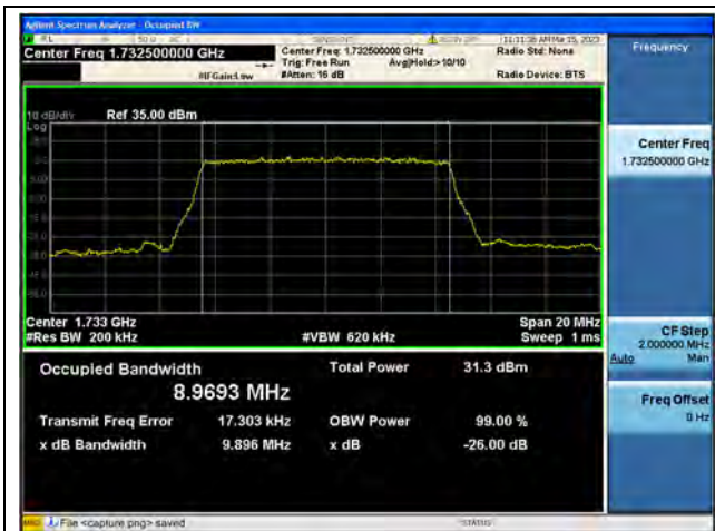
Band4 / 10MHz / QPSK/ Mid CH
