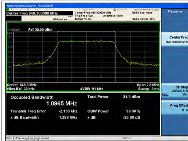
Band5 / 1.4MHz / QPSK/ High CH
