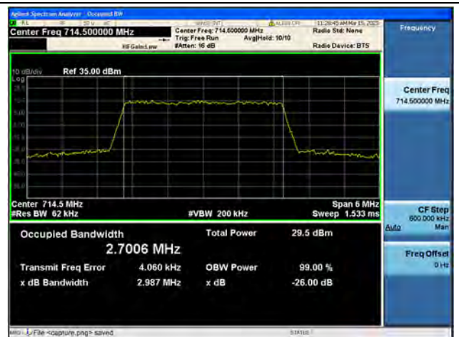
Band12 / 3MHz / 64QAM/ High CH
