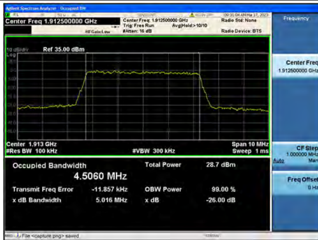
Band25 / 5MHz / 64QAM/ High CH
