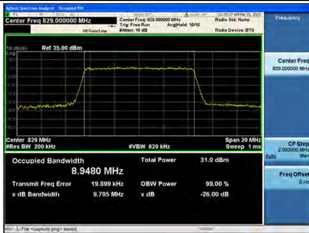
Band5 / 10MHz / 16QAM/ Low CH
