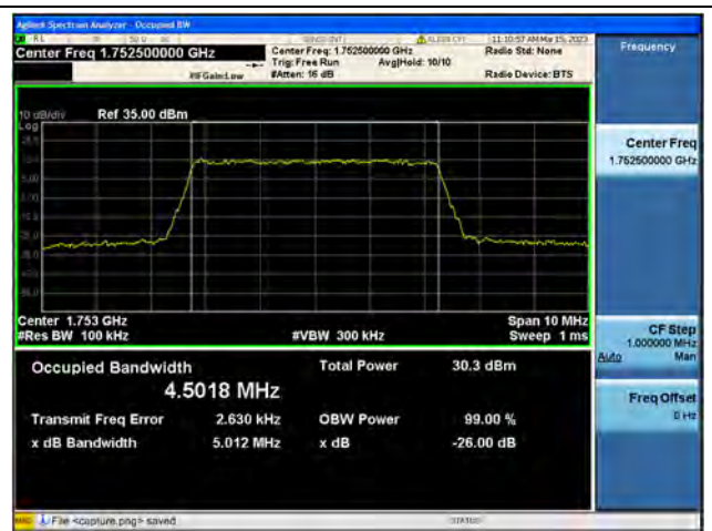
Band4 / 5MHz / 16QAM/ High CH
