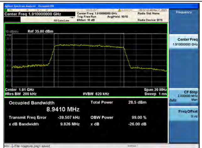
Band25 / 10MHz / 64QAM/ High CH
