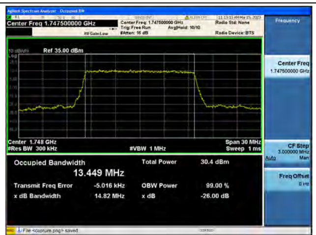
Band4 / 15MHz / 16QAM/ High CH
