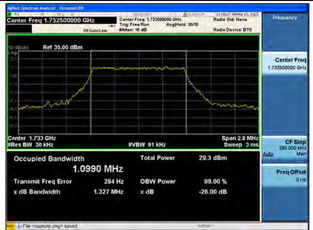
Band4 / 1.4MHz / 64QAM/ Mid CH
