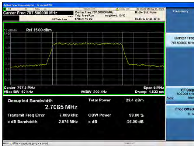
Band12 / 3MHz / 64QAM/ Mid CH
