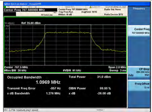
Band12 / 1.4MHz / QPSK/ Mid CH
