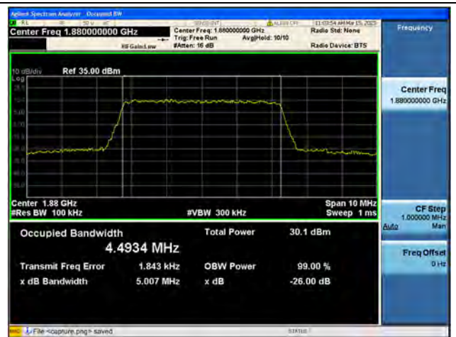
Band2 / 5MHz / 64QAM/ Mid CH
