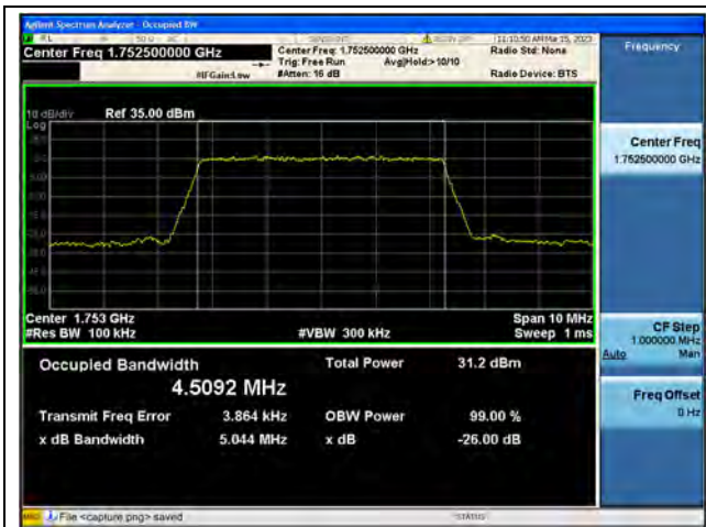
Band4 / 5MHz / QPSK/ High CH
