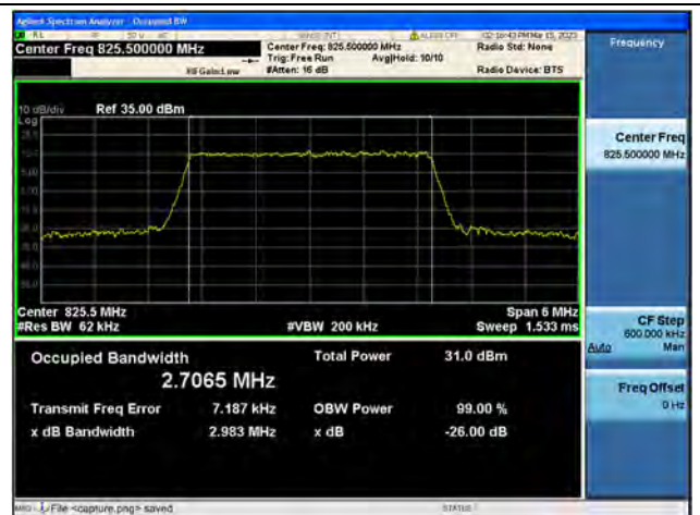
Band26 Part22 / 3MHz / 64QAM/ Low CH
