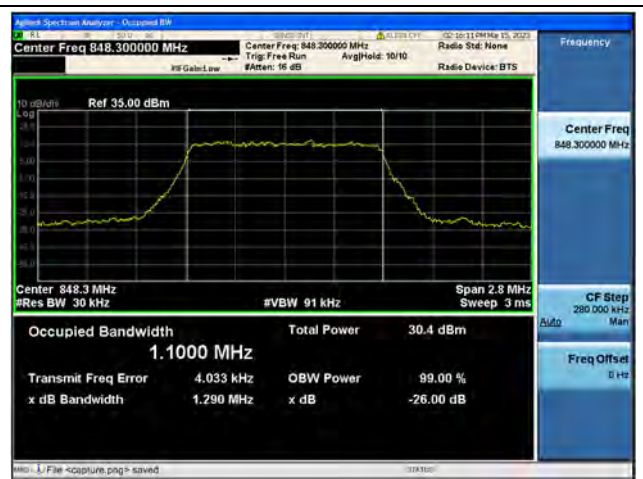
Band26 Part22 / 1.4MHz / 16QAM/ High CH
