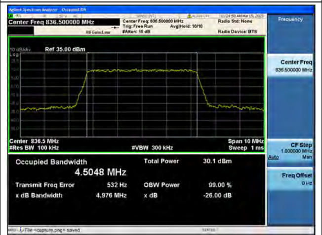
Band5 / 5MHz / 64QAM/ Mid CH
