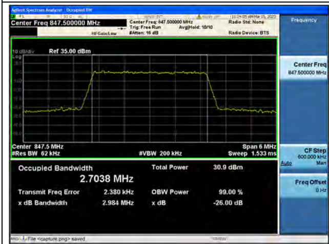
Band5 / 3MHz / 16QAM/ High CH
