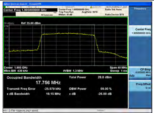
Band25 / 20MHz / 64QAM/ High CH
