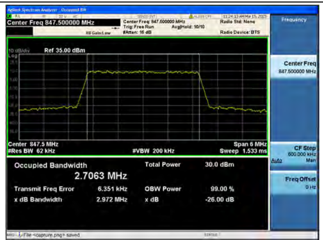
Band5 / 3MHz / 64QAM/ High CH
