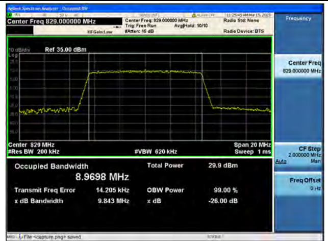
Band5 / 10MHz / 64QAM/ Low CH
