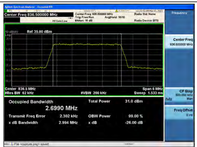
Band5 / 3MHz / 16QAM/ Mid CH
