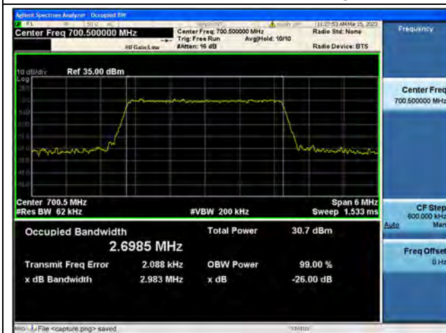
Band12 / 3MHz / 16QAM/ Low CH
