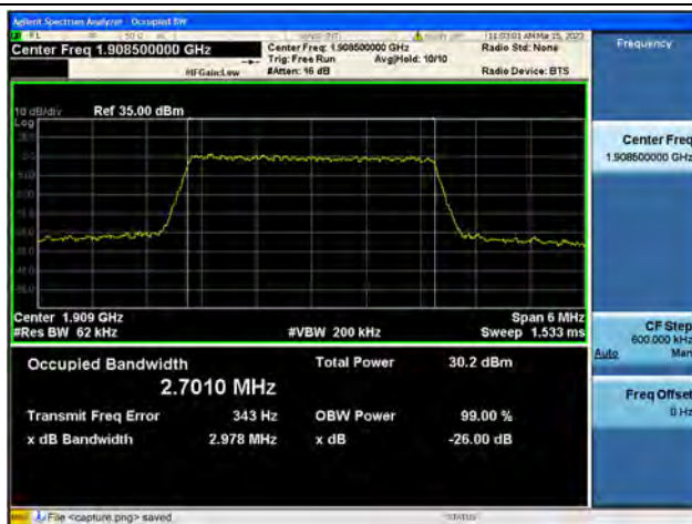
Band2 / 3MHz / 16QAM/ High CH
