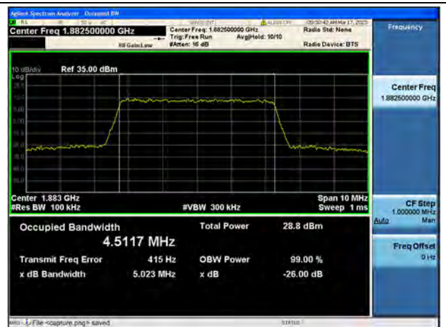
Band25 / 5MHz / 64QAM/ Mid CH
