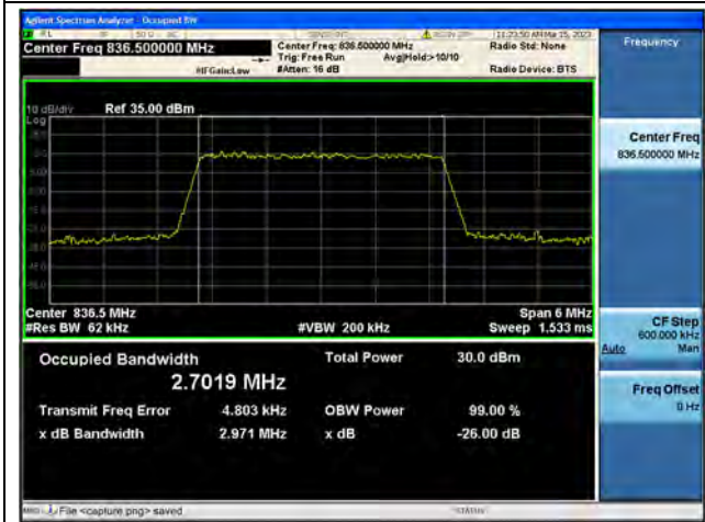
Band5 / 3MHz / 64QAM/ Mid CH
