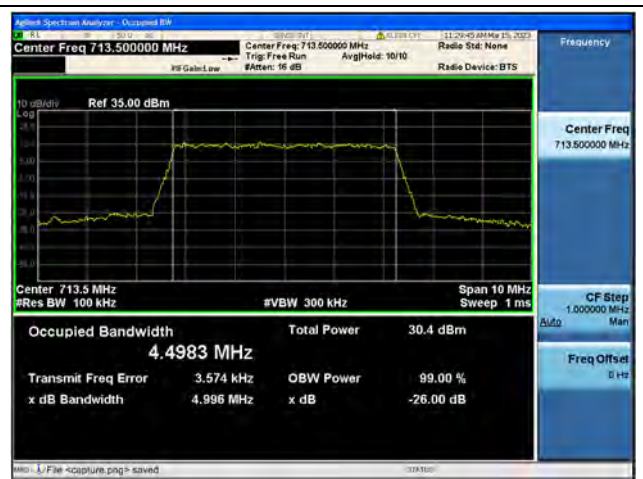
Band12 / 5MHz / 16QAM/ High CH
