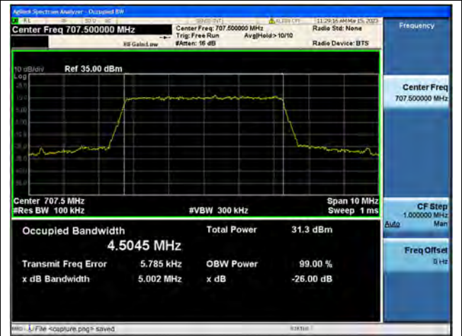
Band12 / 5MHz / QPSK/ Mid CH
