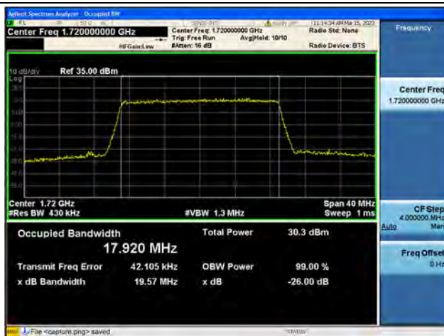
Band4 / 20MHz / 16QAM/ Low CH
