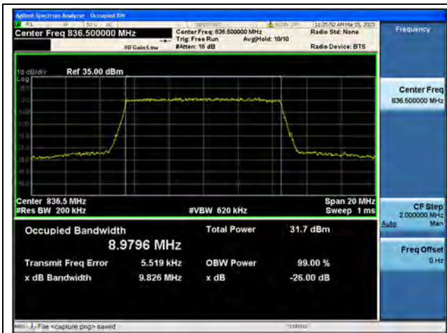
Band5 / 10MHz / QPSK/ Mid CH
