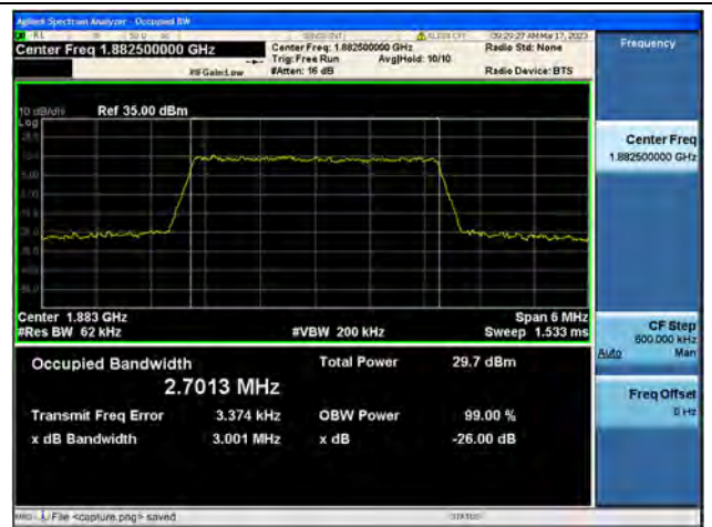
Band25 / 3MHz / 16QAM/ Mid CH
