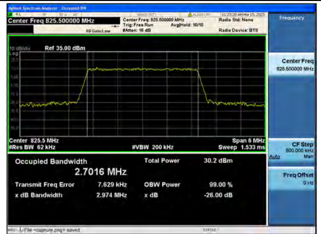
Band5 / 3MHz / 64QAM/ Low CH
