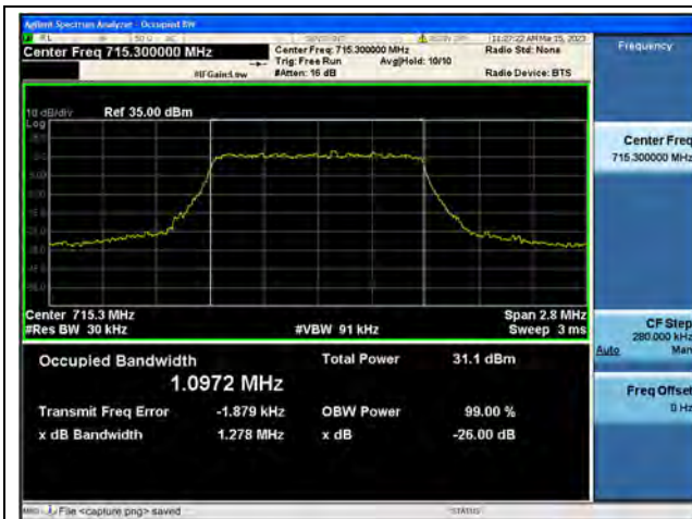
Band12 / 1.4MHz / QPSK/ High CH
