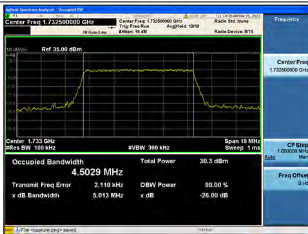
Band4 / 5MHz / 16QAM/ Mid CH
