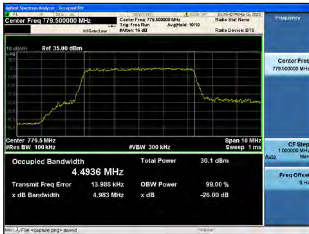
Band13 / 5MHz / 64QAM/ Low CH
