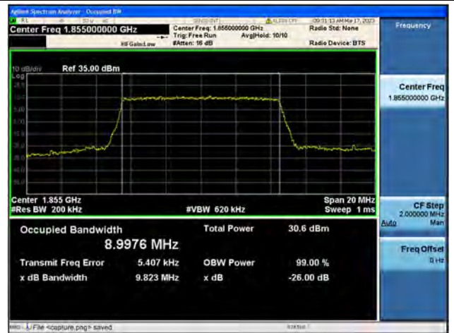
Band25 / 10MHz / QPSK/ Low CH
