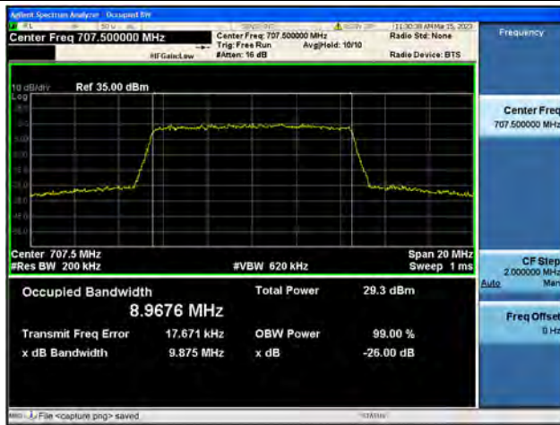
Band12 / 10MHz / 64QAM/ Mid CH
