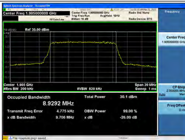
Band2 / 10MHz / 16QAM/ High CH
