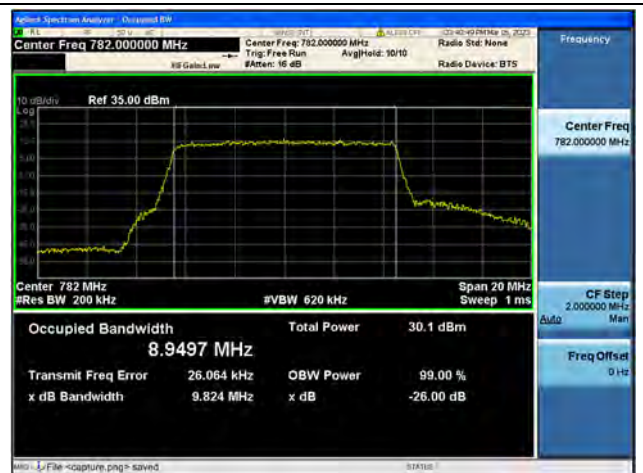
Band13 / 10MHz / 64QAM/ Mid CH
