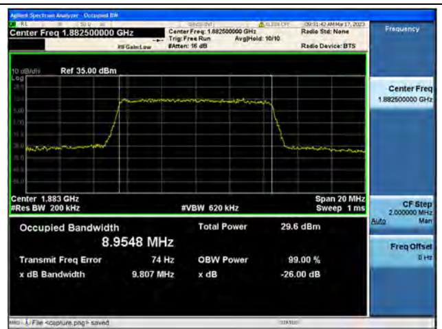
Band25 / 10MHz / 16QAM/ Mid CH
