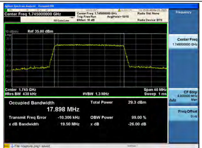
Band4 / 20MHz / 64QAM/ High CH
