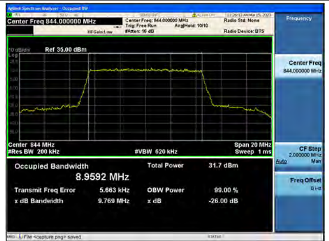
Band5 / 10MHz / QPSK/ High CH
