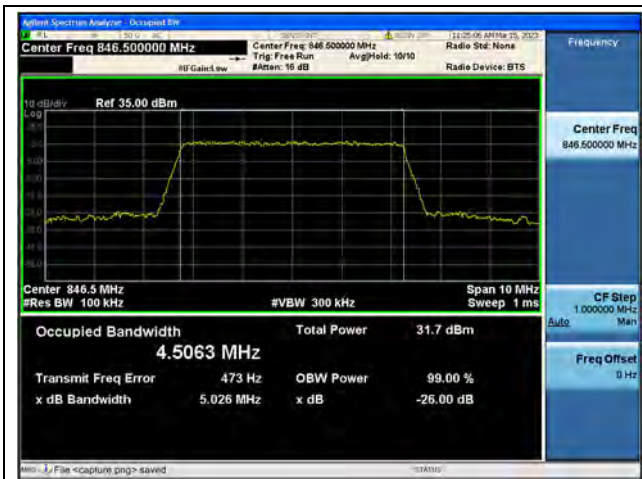
Band5 / 5MHz / QPSK/ High CH
