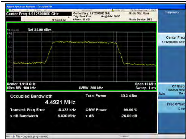
Band25 / 5MHz / QPSK/ High CH
