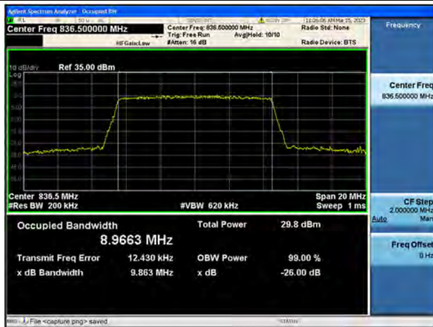
Band5 / 10MHz / 64QAM/ Mid CH
