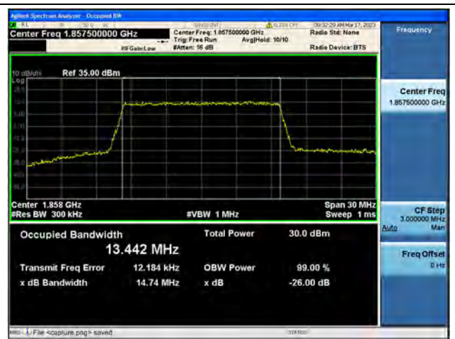
Band25 / 15MHz / 16QAM/ Low CH
