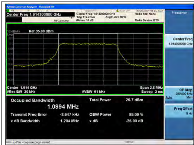
Band25 / 1.4MHz / QPSK/ High CH
