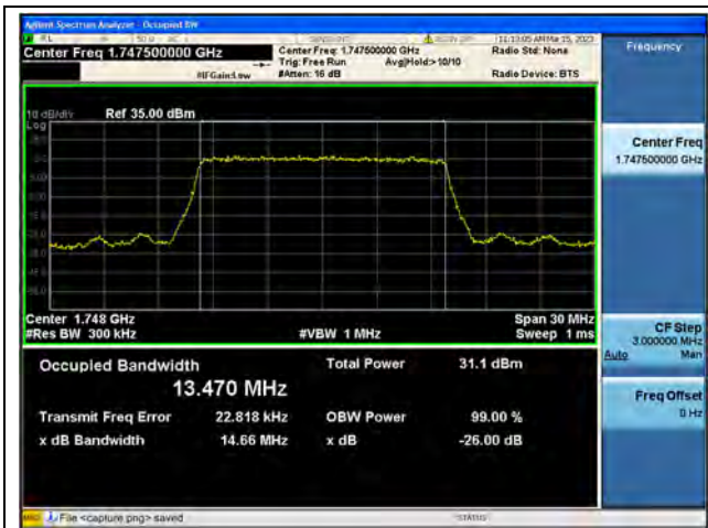
Band4 / 15MHz / QPSK/ High CH
