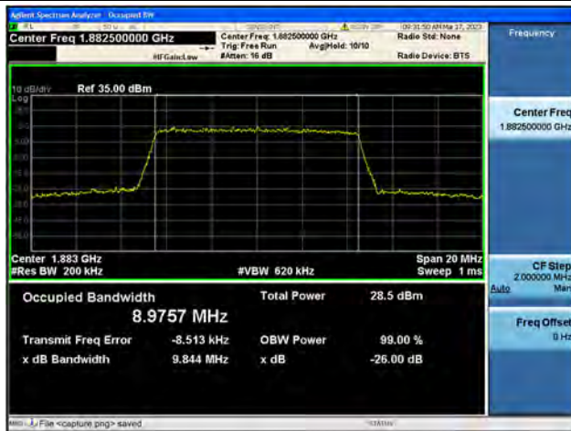
Band25 / 10MHz / 64QAM/ Mid CH
