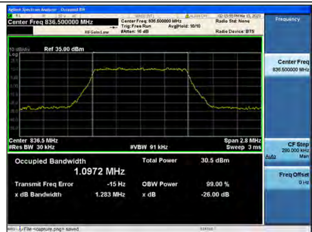
Band26 Part22 / 1.4MHz / 64QAM/ Mid CH
