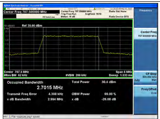
Band12 / 3MHz / 16QAM/ Mid CH
