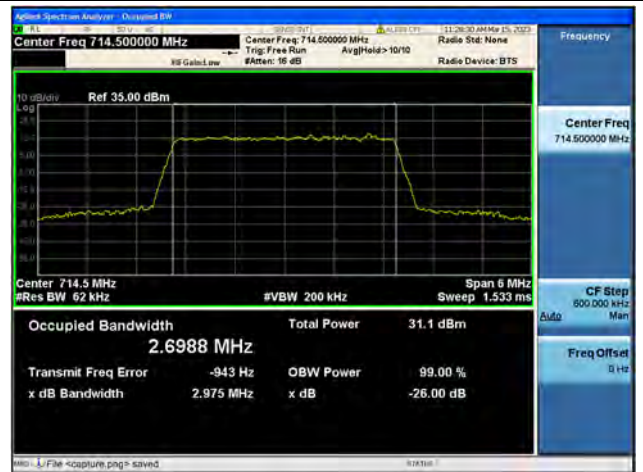
Band12 / 3MHz / QPSK/ High CH
