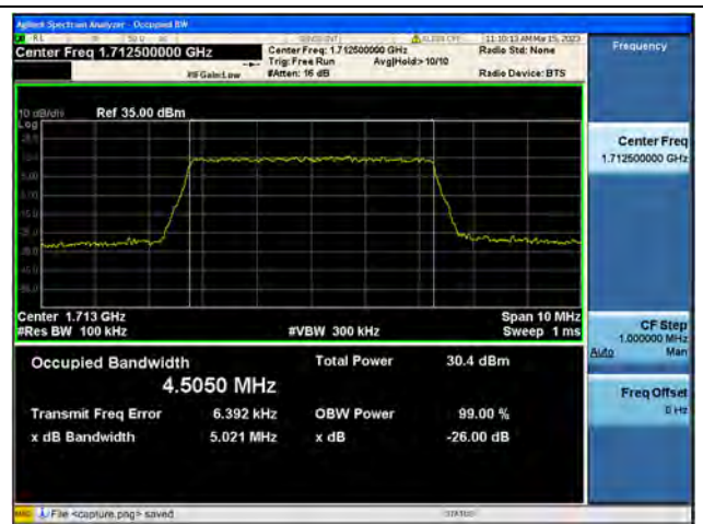
Band4 / 5MHz / 16QAM/ Low CH
