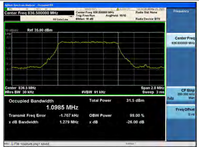
Band5 / 1.4MHz / QPSK/ Mid CH
