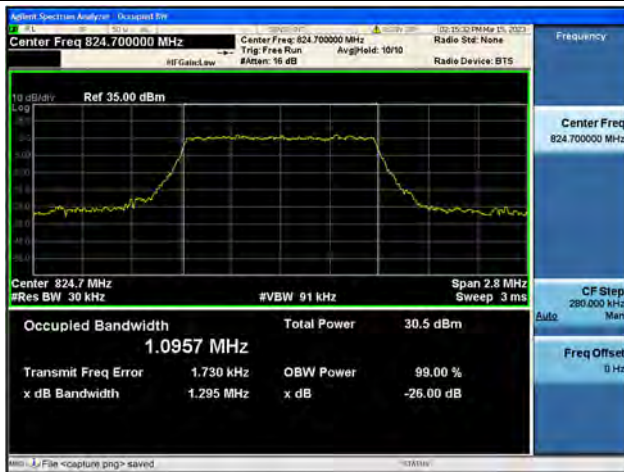
Band26 Part22 / 1.4MHz / 64QAM/ Low CH
