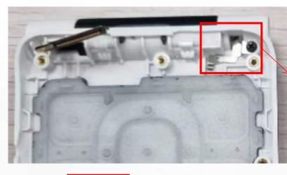
The rotating shaft needs to be properly treated, and the shrapnel should be retained.
