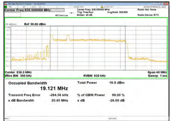
B2_N5(20M)_CP-OFDM_QPSK_Outer_Full_Mid_CH
