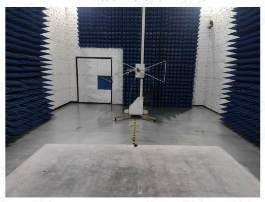
RADIATED EMISSION TEST SETUP ABOVE 1GHz
