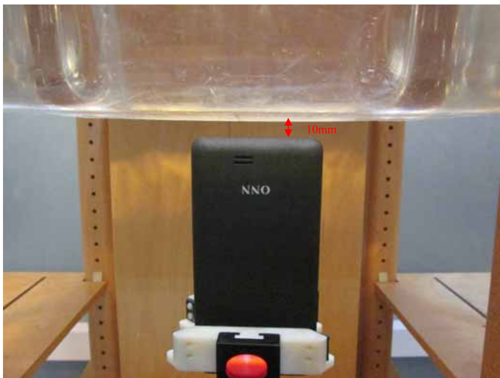
Body-worn Bottom Setup Photo (10mm)
