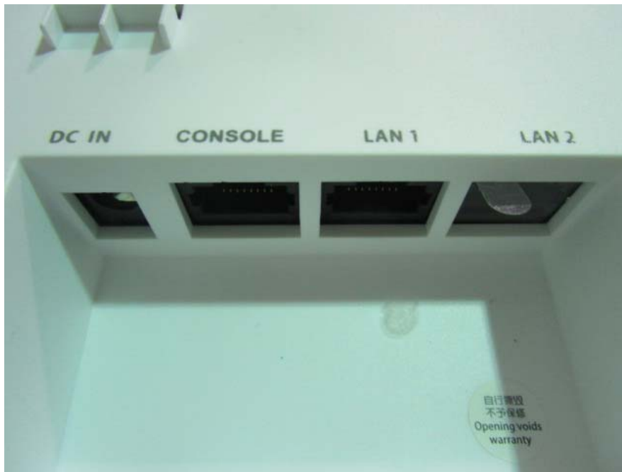
EUT – Ports View
