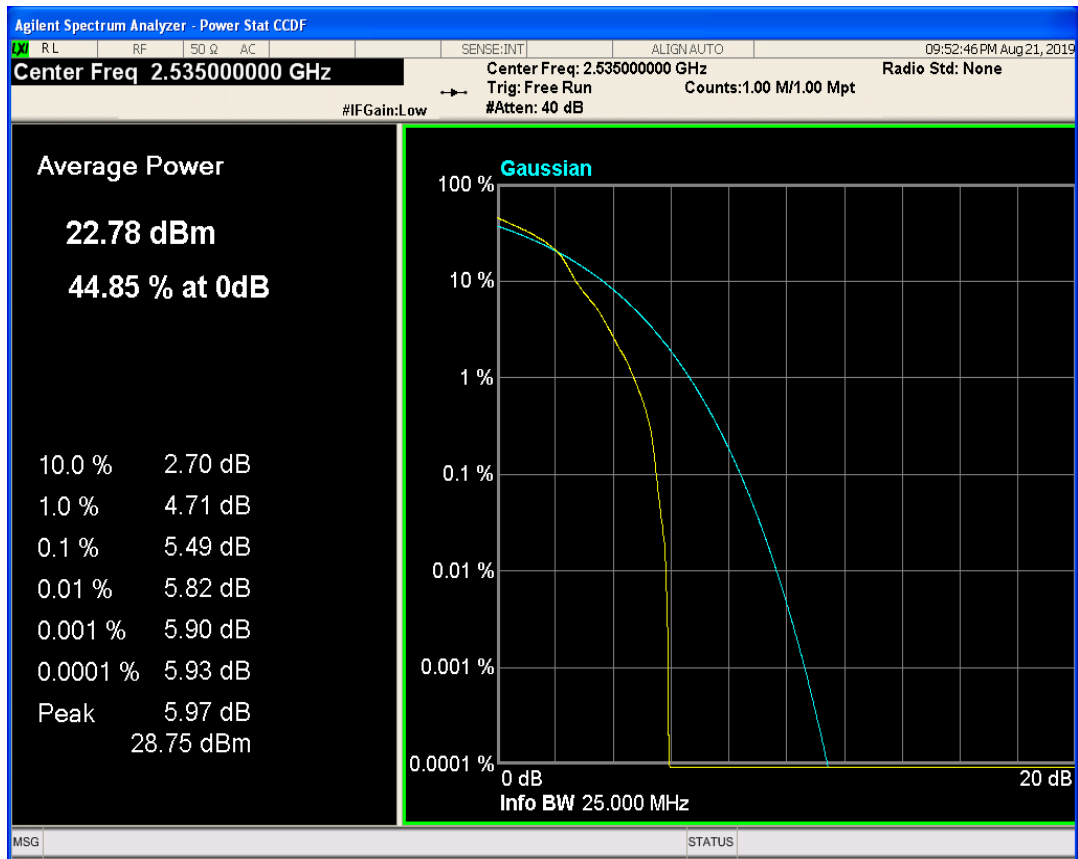
LTE Band7 QAM16 BW=20MHz Channel=21100 RB Size=1 Position=#0
