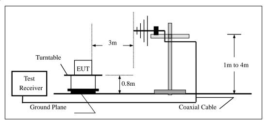
(c) For radiated emissions above 1000MHz
