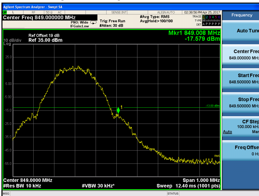
Higher Band Edge Plot on Channel 251
