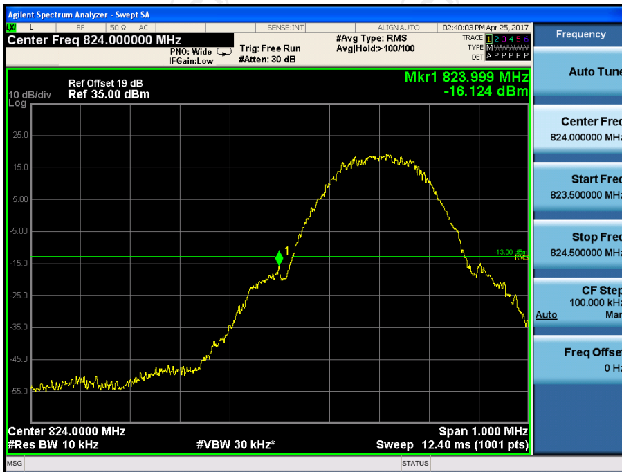
Higher Band Edge Plot on Channel 251
