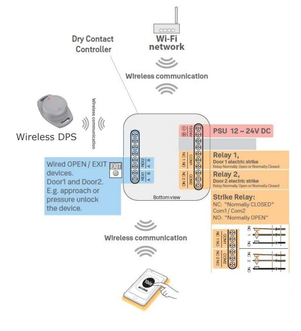
Sahara is a dry contact device that is built with Wi-Fi and Bluetooth connections that allow the Yale Access app to send an electric strike to a GDO (Garage door opener) or Gate automation device that is it connected to.
