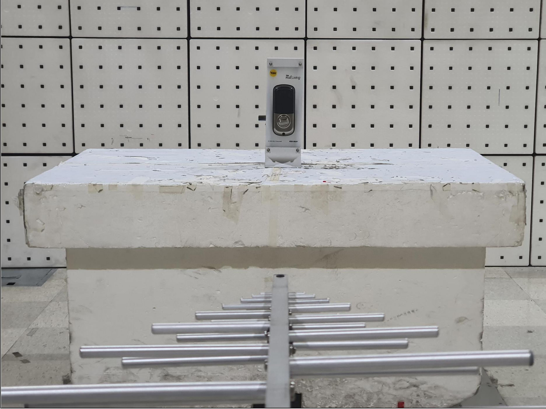
Radiated Emission (Below 1 GHz) _ Rear_ (Test Model : YRD137)
