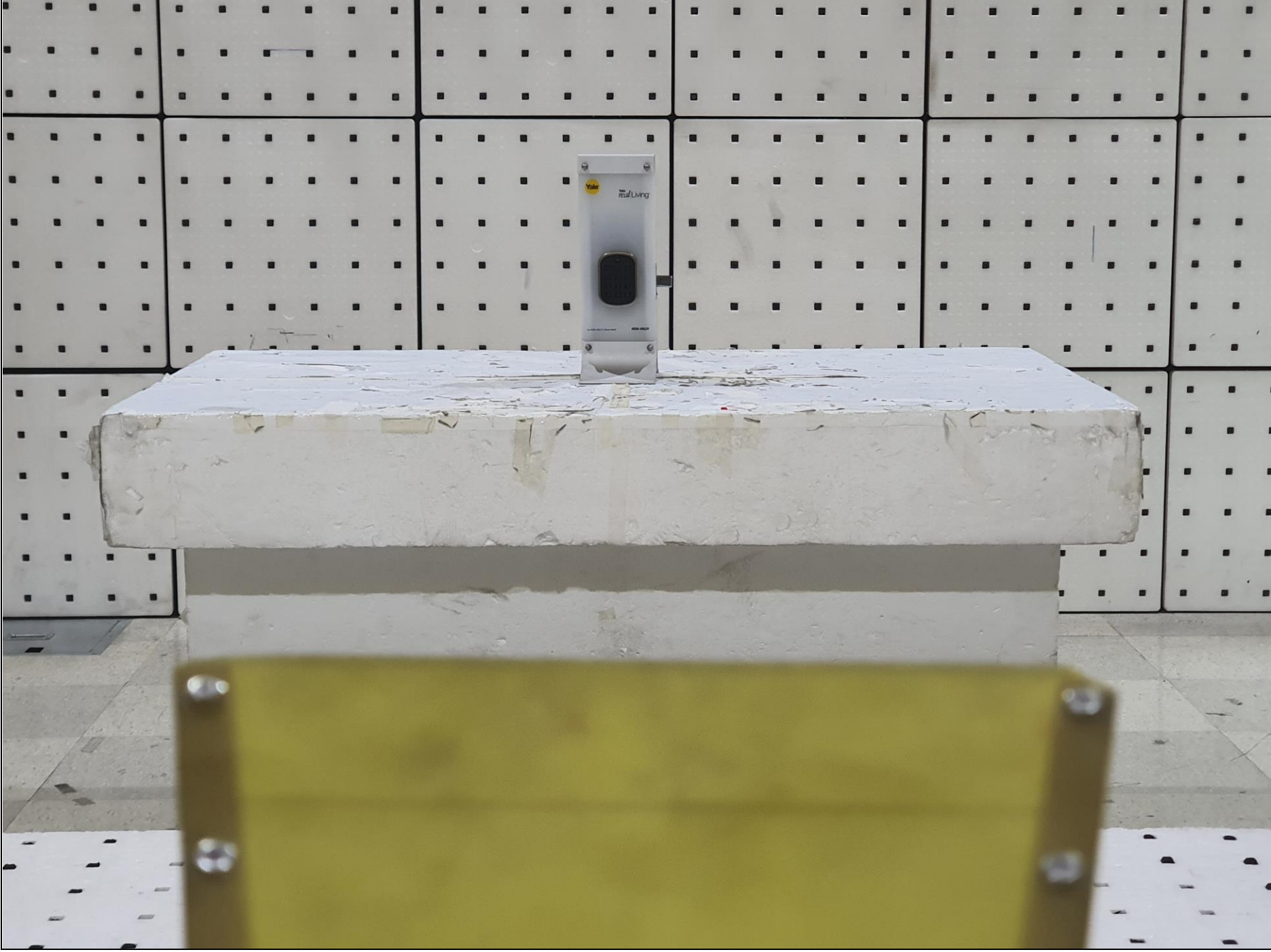
Radiated Emission (Above 1 GHz) _ Front_ (Test Model : YRD137)
