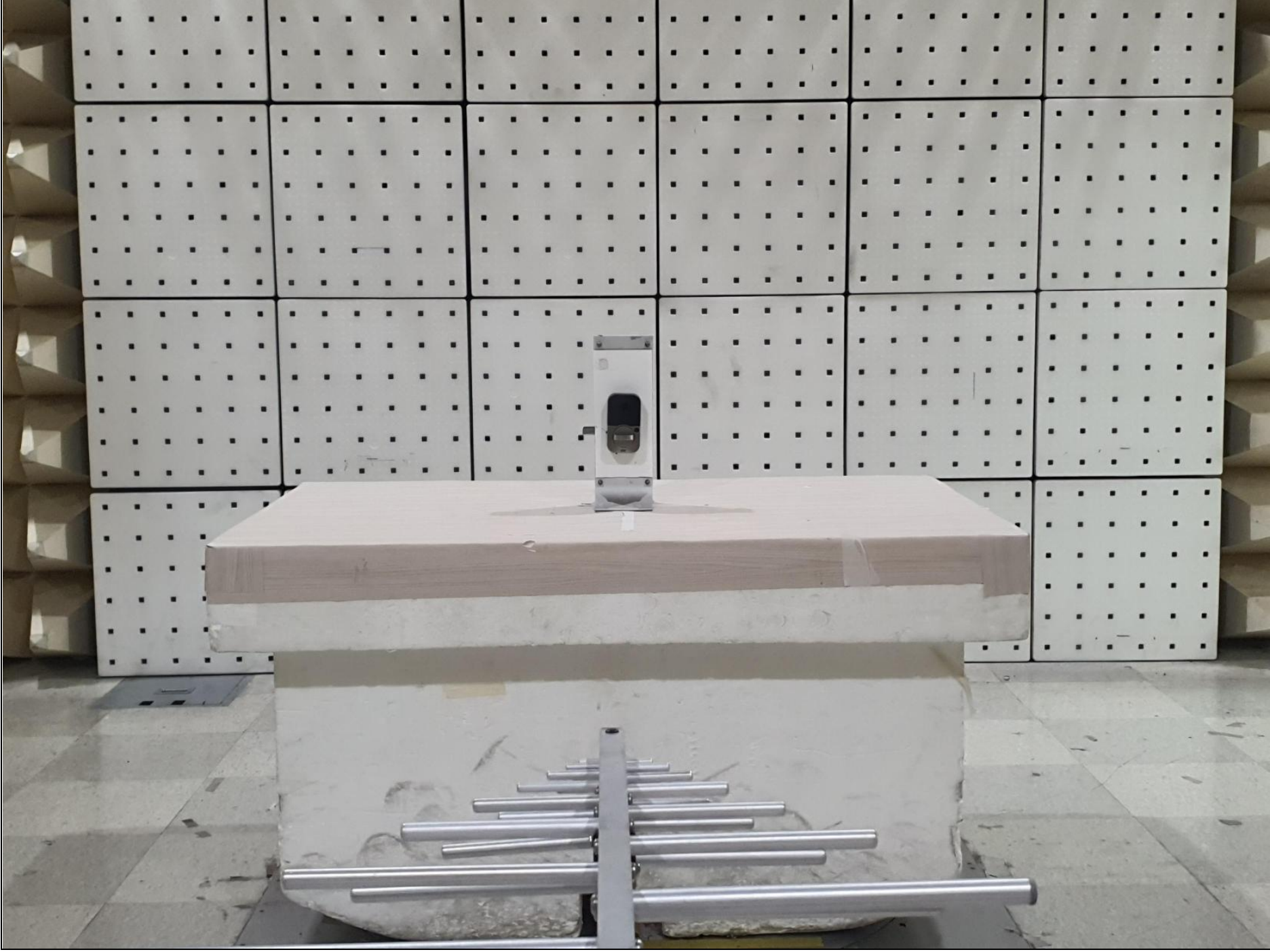
Radiated Emission (Below 1 GHz) _ Rear [Basic Model : YRD450 FP]
