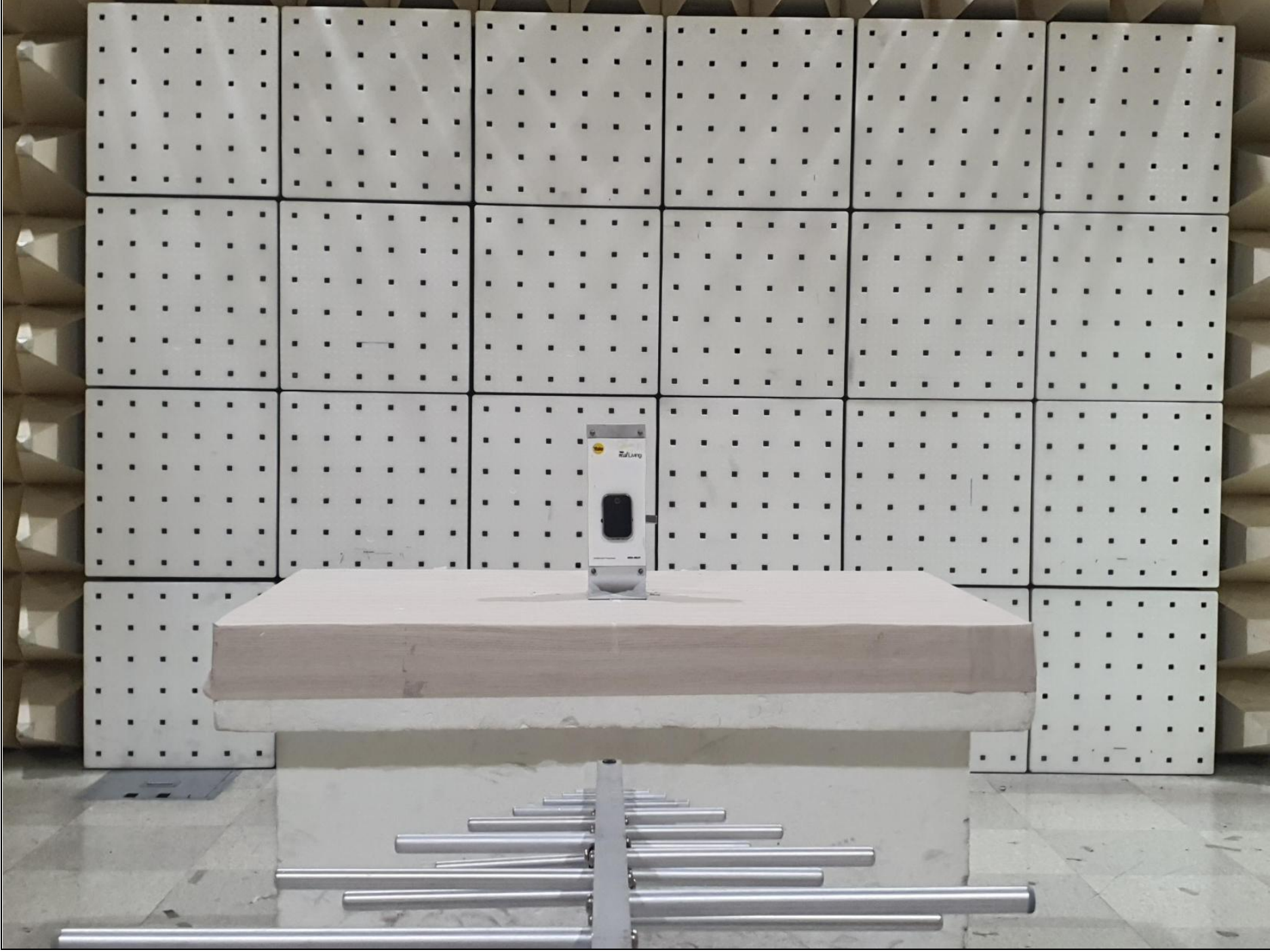
Radiated Emission (Below 1 GHz) _ Front [Basic Model : YRD450 FP]
