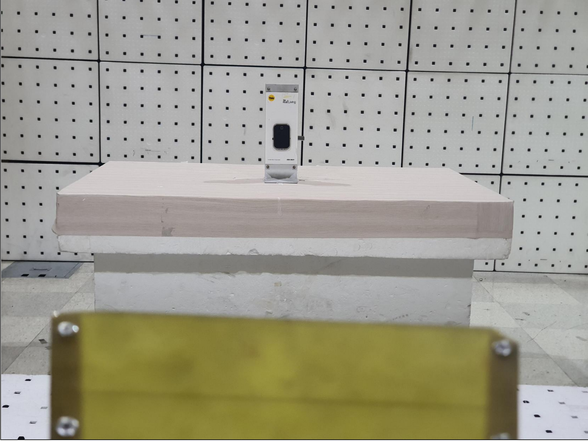
Radiated Emission (Above 1 GHz) _ Front [Basic Model : YRD450 FP]
