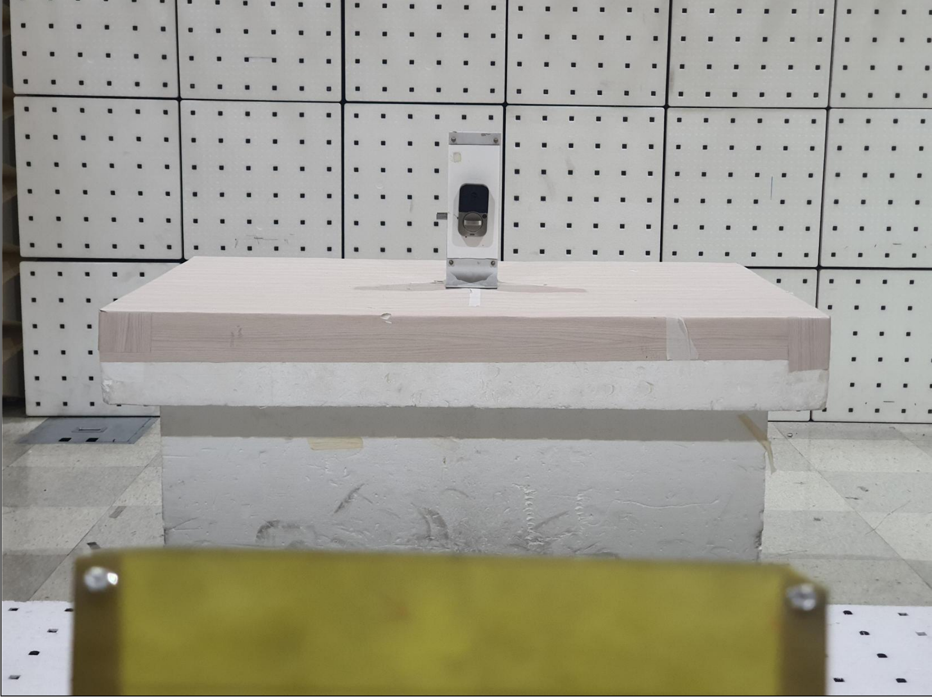
Radiated Emission (Above 1 GHz) _ Rear [Basic Model : YRD450 FP]
