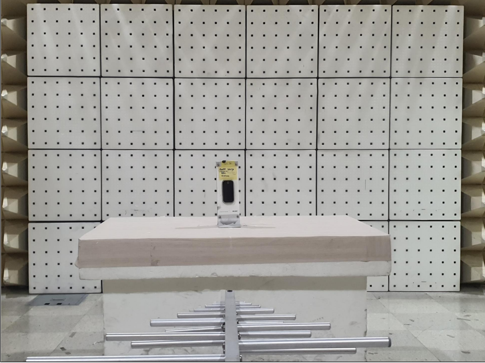
Radiated Emission (Below 1 GHz) _ Front [Alt. Model : YRD420 FP]
