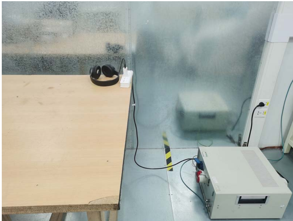
Conducted Emission Test Setup:
