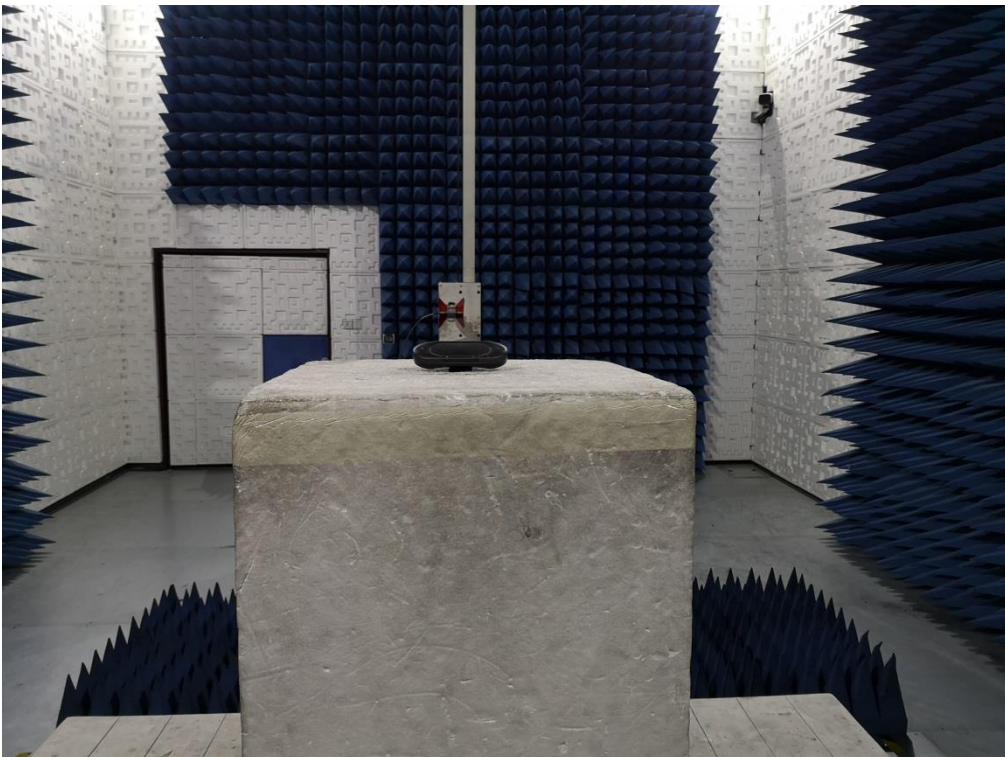
RADIATED EMISSION TEST SETUP ABOVE 1GHZ
