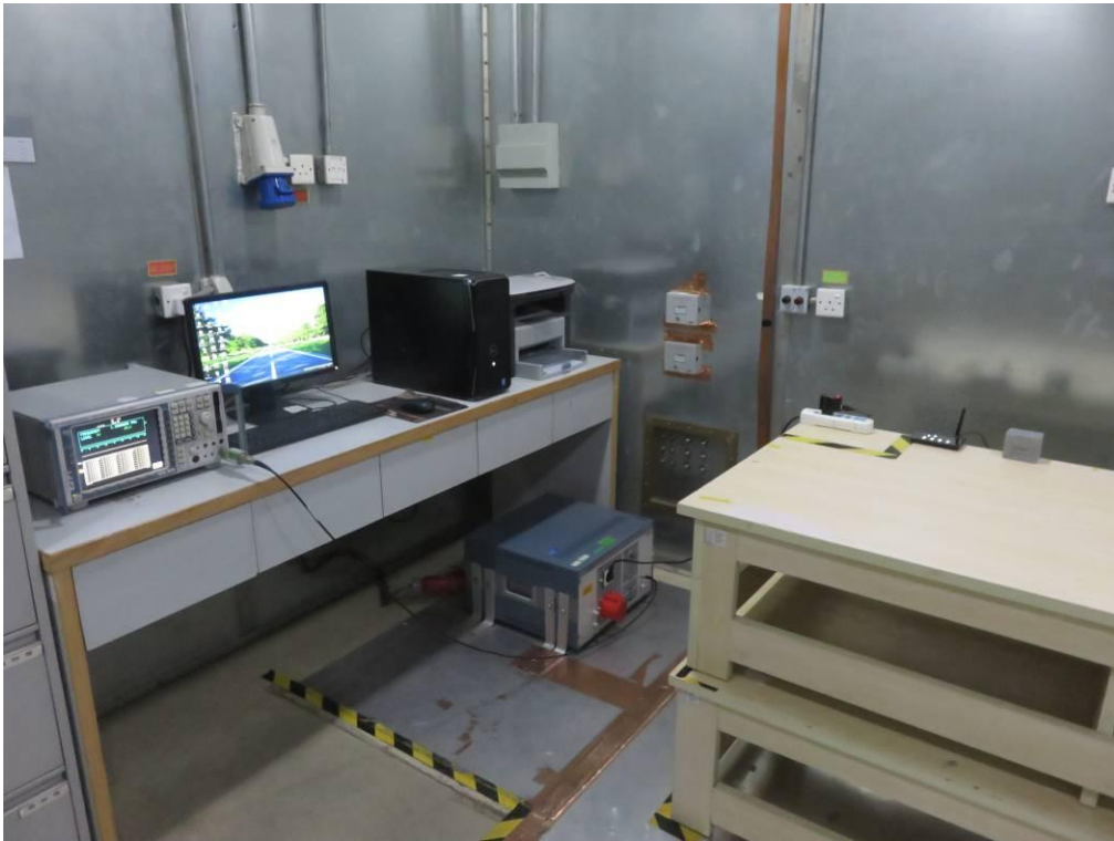
FCC RADIATED EMISSION TEST SETUP
