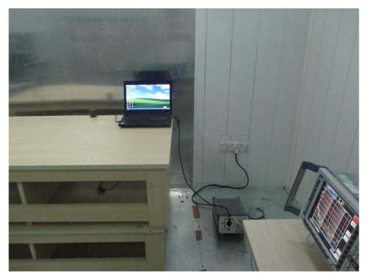
FCC RADIATED EMISSION TEST SETUP
