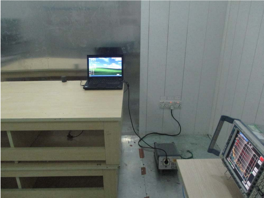
FCC RADIATED EMISSION TEST SETUP
