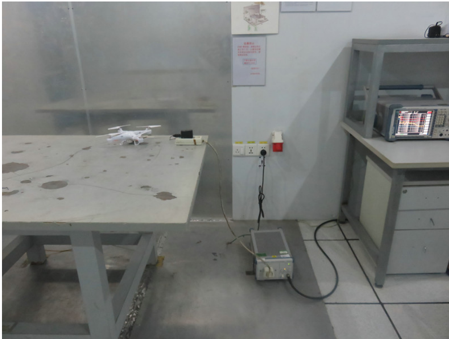
6.1. Photo of Conducted Emission Measurement
