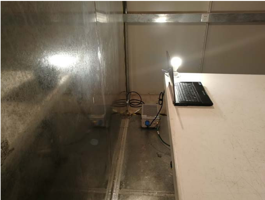
Conducted Emissions (Side View)
